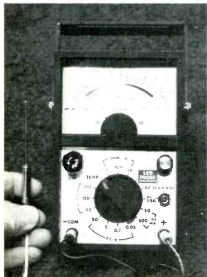
Fig. 7 The metal thermistor probe is waterproof. Temperatures from about 60°F to 500°F can be measured.
