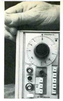
Fig. 2 The Tektronix SG-502 audio generator produces low-distortion sine waves and sharp square waves.
