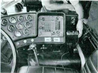
Fig. 1. In many trucks, a CB radio might interfere with movements of the driver's leg, if mounted under the dash in the usual way (left). Sometimes sufficient room can be found around the center console of a cab-over-engine model (right). Be sure the space isn't needed for something else, and that the driver can reach the CB controls and hear the speaker.
