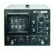
Vertical-deflection sensitivity has 11 ranges between .01 volt-per-centimeter and 20 volts-per centimeter.
