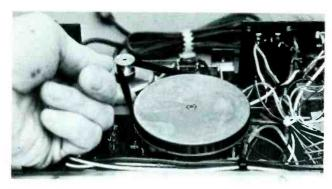
Step 4. The motor pulley drives a rubber belt (usually flat). The belt wraps around and spins the heavy, speed-smoothing flywheel. If the belt is dirty, worn, or stretched, it can slip on the motor pulley and allow slow or erratic tape movement. Severe looseness might prevent the belt from turning the flywheel at all. If the belt is dirty, clean it with isopropyl alcohol. If it's worn or stretched, replace it.
