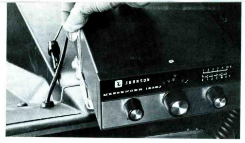
Fig. 8 Thumb nuts and an exposed fuse holder allow the driver to remove the CB rig quickly, if necessary to foil would-be thieves. Use grommets in every hole where wires must pass through.
