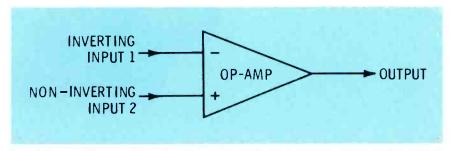
Fig. 1 This is the usual symbol for an op-amp. The polarity signs at the inputs do not refer to the DC voltage, but indicate the polarity of signal at the input which gives a positive-going output signal.
