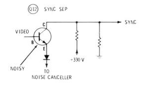
Symptom—Noise in picture, radiates to other sets Cure—Check Q12, or replace it on suspicion
