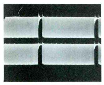
**Fig. 6** Evidently blanking is applied to the 3.58-MHz demodulator signals (scope at horizontal scanning rate) rather than to the chroma signal. The R-Y carrier at W27 and the B-Y carrier at W25 both have same amplitude (1 volt PP) and waveshape, but different phase.
