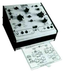
The Hickok Model 440 semiconductor curve tracer is all purpose and convenient to use. It's the ideal instrument for testing, evaluating, classifying and matching all types of transistors, FET's and diodes. You'll get stable, full range dynamic displays that you can accurately scale right from the screen.
