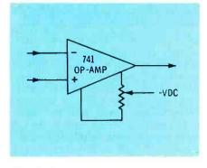
**Fig. 7** Some op-amps, such as the 741, provide external terminals for offset nulling.
