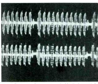
Fig. 4 These waveforms are nearly identical except for amplitude. At the top is the .6 volt PP bar signal at module U14 (point "Q"); and the .24 volt PP signal at the bottom was found at pin 13 of IC1001.
