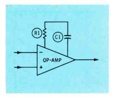
Fig. 8 Not all op-amps have internal frequency compensation. Some have terminals for external compensation. This circuit is for compensation of the input stages; others compensate the output stage, also.
