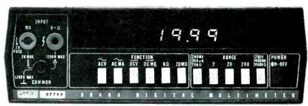
Resolution is 100 microvolts, 100 nanoamps and 100 milliohms
