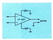
Fig. 2 For those applications where zero output (offset) voltage is required in the absence of input voltage, two identical power supplies of opposite polarity are necessary. AC amplification is possible from a single supply, if input and output coupling capacitors are used.
