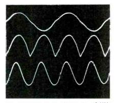
Fig. 5 The top trace shows the 19-KHz sine-wave signal from Q302. 38-KHz parabolas are formed by rectification at the common cathodes of the diodes (center trace), and after amplification and filtering, the parabolas become 38-KHz sine waves (trace at bottom) ready to demodulate the sidebands.
