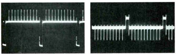
Fig. 6 Similar sync compression and increased ringing also can be seen in the scope waveforms of lines. In the left waveform, the signal is 10 vertical lines at the horizontal scope speed. It's negative-going video that's fed to a video stage. After passage through two video amplifiers, the sync is compressed and the spikes representing lines have excessive ringing (right waveform). This set was normal; do the same test with other receivers, and you soon will know how much change is normal.
