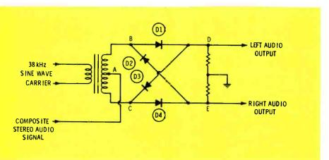
Fig. 3 Diode-type synchronous demodulators greatly simplify the new circuits by not requiring separation of the L+R and L-R signals. Two basic actions take place here: the correctly-phased 38-KHz carrier is inserted into the L-R sidebands to form the original L-R signal, by diode demodulation; also the L+R audio (a part of the composite audio) combines with the L-R audio to provide true left and right stereo audio signals.
