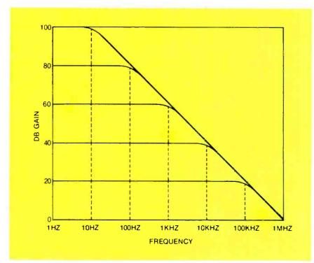
Fig. 3 Frequency compensation to make the gain stable and without self-oscillation severely attenuates the high frequencies. Then external negative feedback is used to flatten the response. The 741 can be made to have flat response up to 1 MHz if the gain is reduced to 1.
