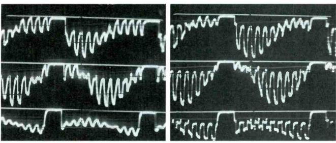
Fig. 8 Waveforms at the cathodes of the picture tube are different with video. Picture at left shows bars without video. Top trace is 60 volts PP red signal, center is 65 volts PP blue signal, and bottom is 24 volts PP of green cathode signal. Waveforms of the right picture are the same except the video (dark spaces between the bars) is included.
