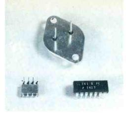
741 op-amps in two different forms are in the foreground, and the power transistor gives an idea of the op-amps small size.
