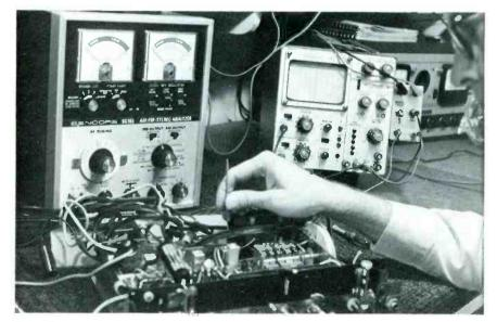
**Bob Goodman** tweaks an adjustment in the multiplex circuit of an AM/FM-stereo radio receiver.
