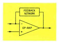
Fig. 4 Phase of the signals at the output and the inverting input are correct for negative feedback; the network is placed between them. The signal input can be either at the inverting input or the non-inverting input, as desired.
