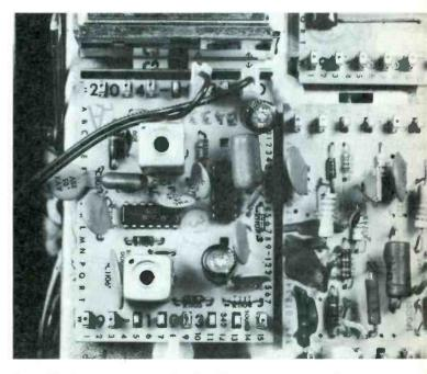
Fig. 10 On the left is the 9-103 audio module. The power-amplifier IC (IC1102) is the one on the right. IC1101 (IF amplifier, detector, and low-level audio) is at the left.
