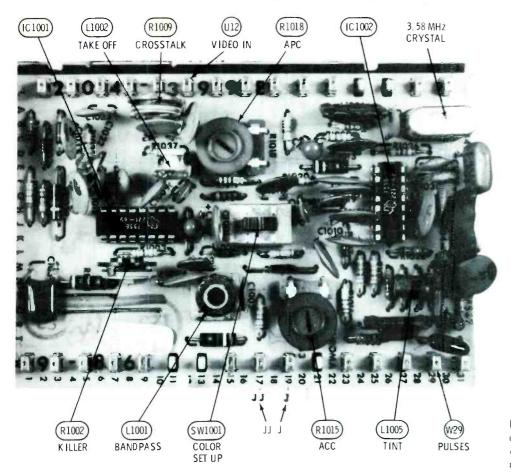
Fig. 1 Locations of major components and adjustments on the Zenith 9-86 chroma module are shown.
