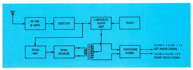
Fig. 2 Without the bandpass tuned amplifiers of the older multiplex circuits, the block diagram of a modern FM-stereo radio is not complicated.
