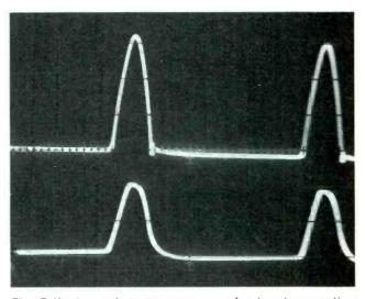
Fig. 7 Keying pulses are necessary for burst separation (and carrier blanking?). Top trace shows 7 volt PP horizontal pulses at W29; and 4 volt PP pulses at 1C pin 4 are at the bottom.
