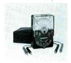
Voltage sensitivities are 20,000 ohms-per-volt DC and 10,000 ohms-per-volt AC. The unit is built with two silicon diodes for meter overload protection.
