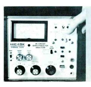
This Hickok Model 220 In-Circuit Semiconductor Analyzer identified all the leads of the germanium PNP transistor, and showed a beta of 200. FET's, SCR's and other devices can be tested, also. Other functions test the resistances of the circuit, and the leakages of transistors and diodes.
