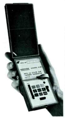
The Hickok Model 239 color bar generator has an exclusive MOS LSI chip which provides 9 Rock Stable patterns and low battery drain.
