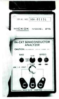
The pocket-sized Model 215 operates on two internal 9-volt batteries, gives a GOOD or BAD readout with LED's, indicates PNP or NPN, and identifies the base (or gate) lead.
