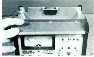
A hinged top with a magnetic catch covers a compartment for storing the power cable and the test leads.
