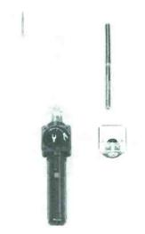
With the new kit installed, a modified probe is capable of testing the HV of all existing b/w and color TV sets. Price of the kit is \$14.50.
