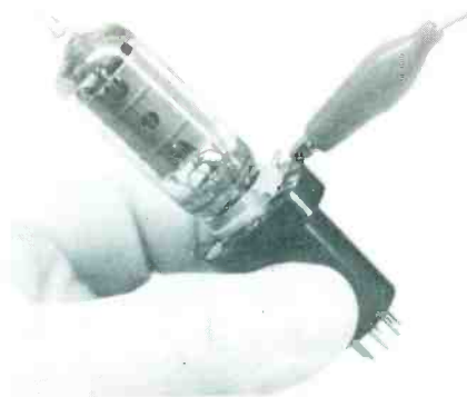
Fig. 5 Socket extenders feed the wiring on through from plug to socket, and provide a lug for each pin so readings can be taken in-circuit. Connect a test lead between each lug in turn to the corresponding point on the circuit board to check for opens.
