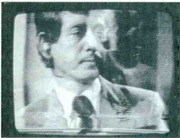
Fig. 2 A more-severe overload than that of Figure 1 might show an image of the other program. Notice the negative image of a woman's face just to the right of the man.
