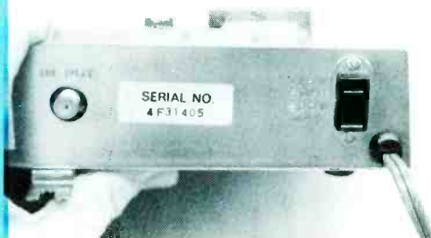
Fig. 3 An AC socket on the rear of the converter supplies switched power for the receiver.
