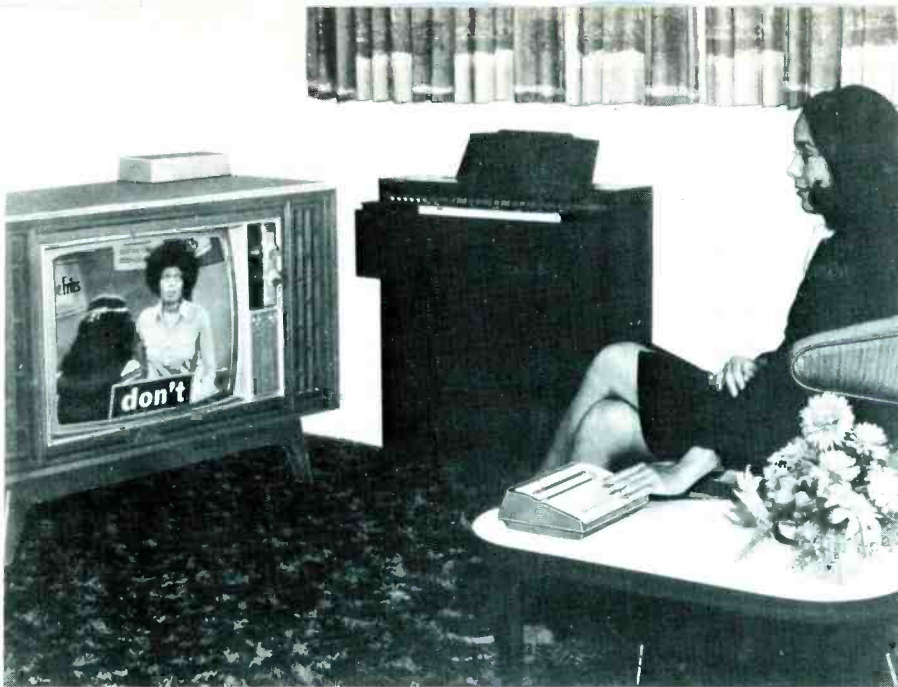
Fig. 1 The Jerrold TRC-12 remote control easily can be installed on any television receiver. Converter and pushbutton remote units are connected by a 25-foot cable. (Courtesy of Jerrold)
