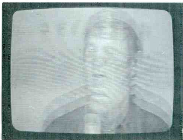
Fig. 4 Sync clipping in a single-channel amplifier might cause the vertical locking to flip.
