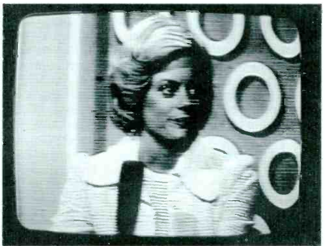
Fig. 3 Excessive input signal, that overloaded a single-channel amplifier, might cause clipping of the sync tips, thus fooling the AGC into increasing the contrast too much.
