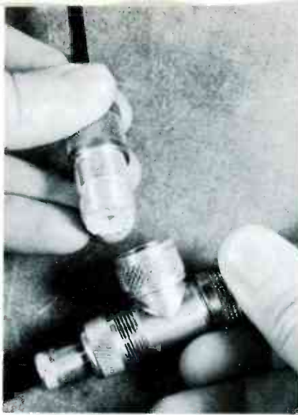
Fig. 5 "T" connector and feedthrough make connections between pulse generator and signal generator for testing effectiveness of noise blanker. Lacking a pulse generator, you can substitute the noise pickup from a piece of wire placed near the running engine of an auto.
