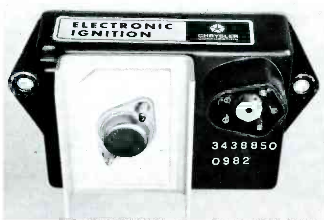
Electronic-ignition subchassis used in the 1972 Chrysler cars. The five-pronged plug is held in place with a screw.
