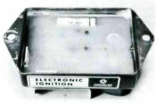
Back side of the Chrysler electronic-ignition unit shows by the components embedded in epoxy that it is non-repairable.
