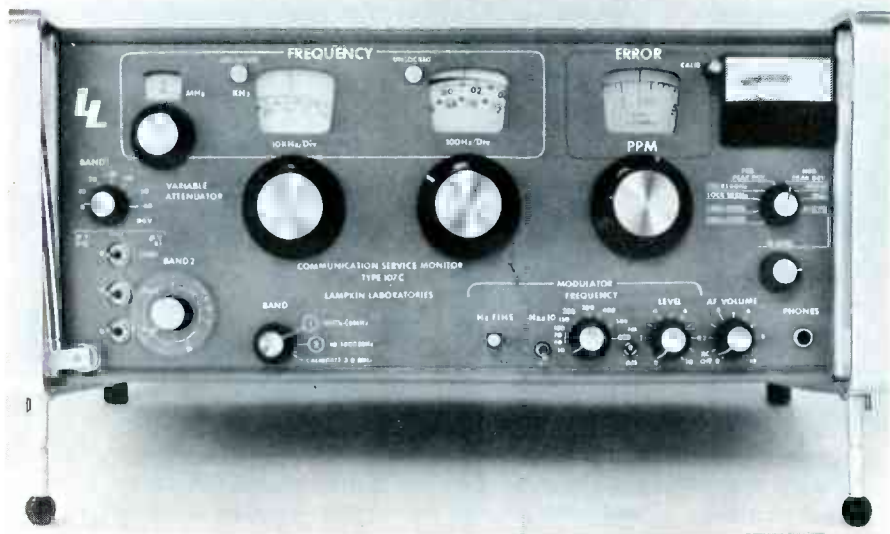
Lampkin 107C has continuous-tuning dials.
