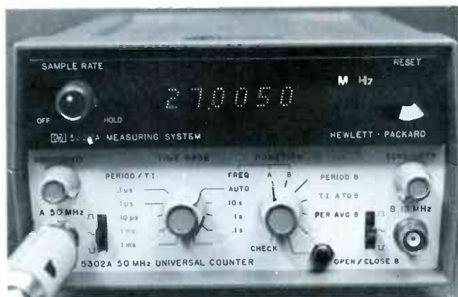
Fig. 8 Digital-readout counter may well become the most popular frequency meter for Citizens Band servicing. It has the advantage of simplicity of operation and virtually immediate indications.
