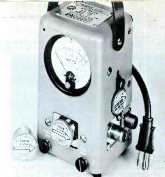
Fig. 3 Peak-reading wattmeter enables technician to measure power of single-sideband transmitter directly. You just talk into microphone during the test. Changeable elements cover many power and frequency variants. For CB, 25-watt 30-MHz element is enough.
