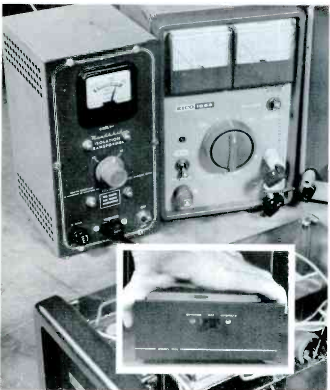
Fig. 2 Bench power supplies should be adjustable, whether for AC (at left) or DC (right). This proves helpful in air-testing any finished repair; intermittents often show up during under- or over-voltage. Inset shows 12-volt supply for turning mobile into base.
