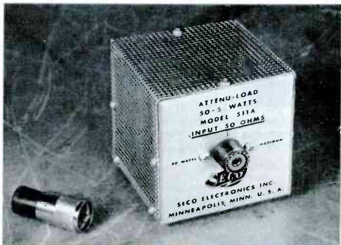
Fig. 4 Single-resistor 50-ohm dummy load at left overheats if you apply 4 watts of CB energy to it continuously. The larger unit, better for bench work, can stay cool handling up to 50 watts of RF.
