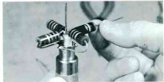
Solder outer leads of 150-ohm resistors to shell of PL-259. Arrange as shown. Center wire is a direct output connection; 10K resistor prevents overloading test instrument (for example, frequency counter) input.
