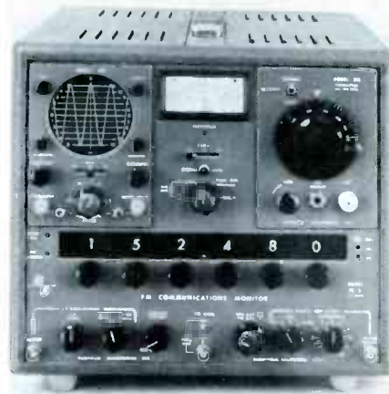
Cushman CE-3 has switched frequency segments.
