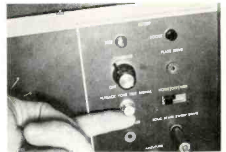
Fig. 5 Inductance-test jack and knobs on model 1077B for checking yoke and transformer when substitution won't work.
