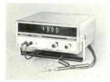
Specifications: Input impedance is 1000 megohms on the 2 volt range, and 10 megohms on the higher ranges. Accuracy of reading of 0.2 per cent on the DC scales can be obtained by use of the DC calibrator, which is furnished preassembled. Accuracy can be increased to 0.1 per cent by calibration against laboratory
