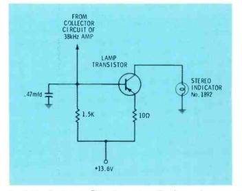
Fig. 6 1971 Ford stereo-FM radios made by Bendix use the stereoindicator circuitry shown here.
