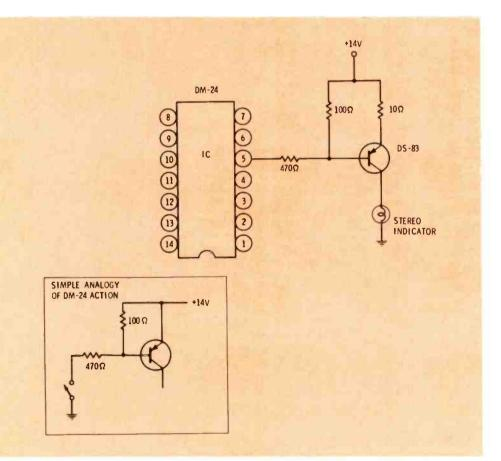
Fig. 8 Both Delco IC's, the DM-14 used in 1970 and the DM-24 used in 1971, use the internal beacon switch of the IC to trigger an external stereo-indicator transistor and lamp. stereo-indicator lamp.
