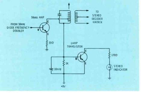
Fig. 4 Stereo-indicator lamp circuitry of a Craig Model 3117 eight-track tape player/stereo-FM radio.
