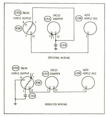
Whenever a failure of the damper heater is found in these early chassis, modification of the wiring is suggested.
