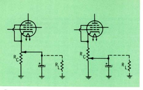
Fig. 4 How a leaky capacitor affects the cathode resistance. (A) Maximum contrast (B) Minimum contrast.
