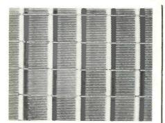
Fig. 7 A low value of R1 in Fig. 2 causes low contrast and a black outline on the right of white objects and a white outline on the right of black objects, as shown here.
