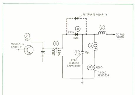
**Fig. 2** The schematic diagram of the video detector of a typical television receiver. The polarity of both the DC and the AC (video) signals is determined by the polarity in which the diode is connected into the circuit.
