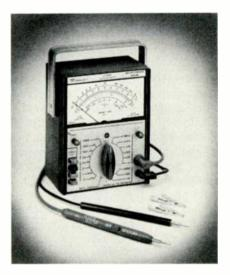
**Decibel ranges:** -30 dB to +62 dB in 8 ranges. Accuracy is  $\pm 3 \text{ per cent on all ranges.}$  Model 603 measures 5½ inches x 6½ inches x 3 3/16 inches, and the weight, with batteries, is 2½ lbs, with one probe, one ground lead, two alli-
