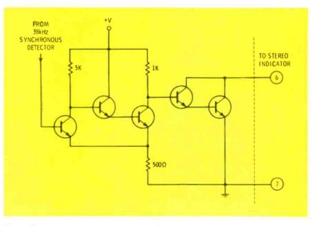
Fig. 11 The two output transistors of the IC's are connected as a Darlington pair, as shown here.
