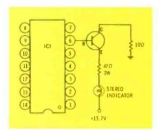
Fig. 9 Motorola Model FM992X stereo-FM car radio uses essentially the same IC stereo-demodulator design circuit as Delco. However, in the Motorola version the lamp switch is connected to pin 6 of the IC.
