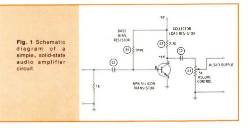
2. Yes. The transistor is not conducting (assuming of course that R2 is not shorted, which is highly unlikely, or that there is a circuit short from the source voltage to the collector, which also is not too likely.)
