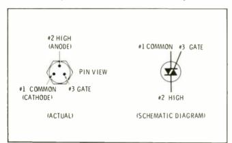
shown here. The triac is used in the on/off function of the remote-control system of RCA CTC54 chassis.
