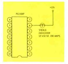
Fig. 10 Becker uses a .030-ampere lamp instead of adding another transistor to handle heavier loads.
