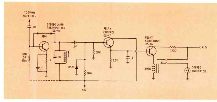
Fig. 1 Stereo-indicator circuit of an early (1965) Delco stereo-FM radio.
