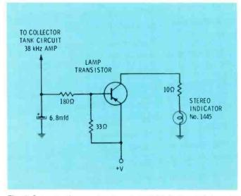
Fig. 5 Stereo-indicator circuitry of 1970-71 Philips (of Canada) auto radios used in Chrysler Corporation automobiles.
