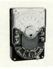
volts full scale; sensitivity is 20,-000 ohms per volt. **5 AC voltage ranges**—5, 25, 100, 500 and 1000 volts full scale; sensitivity is 10,-000 ohms per volt. **4 DC current ranges**—50 microamperes, 5, 50 and 500 milliamperes full scale. **4 resistance ranges**—6K ohms, 600K ohms, 6 megohms and 60 megohms full scale. **5 decibel ranges**—from -20 dB to +62 dB. **Price:** Not available
