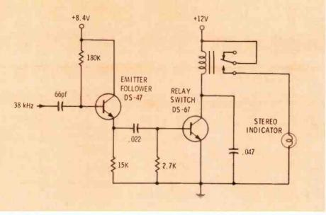
FIg. 2 A third-generation version of the stereo-indicator circuitry used in the 1969 Delco stereo-FM adapter.
