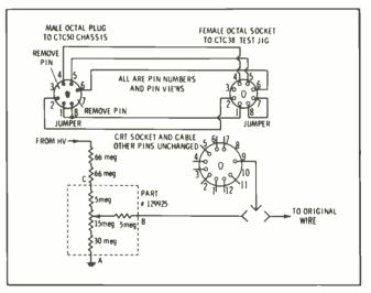
Because the picture tube used with the CTC50 chassis is a low-voltage-focus type, and the picture tube in the test jig requires a focus potential of between 4.6 and 5kV, no raster will be produced by the test jig when connected to the CTC50 unless an external source of sufficient focus voltage is applied to the test-jig picture tube.
