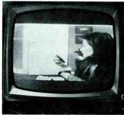
Fig. 10 Shorted turns in the windings of the vertical output transformer or a shorted C39 produces compression or foldover at the top and loss of deflection at the bottom of the raster.
