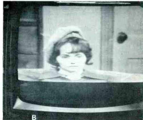
Fig. 9 An open cathode bypass capacitor changes both the deflection and the waveforms. (A) The sawtooth waveform (34 volts PP) obtained at the cathode of V7B when C3C cathode bypass capacitor was opened. (B) On the screen of the picture tube, an open C3C caused a loss of deflection at the bottom of the raster.
