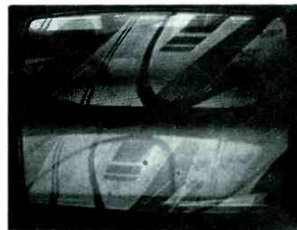
Fig. 6 Lack of sync can be tracked down with substitute sync signal from video generator. (B&K Model 1077B is used to demonstrate technique.) Pattern should lock in with sync injected at any of several points.
