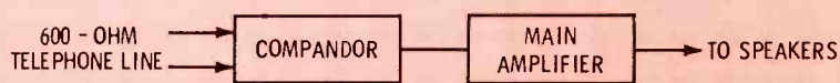
Fig. 24 Compandor, installed between line and amplifier, compresses excessive low-level signals to offset variations in signal level.
