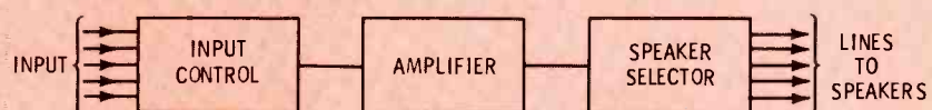
Fig. 3 Block diagram of basic central sound system, which has two or more input signal sources and distributes sound on a controlled basis into various rooms.
