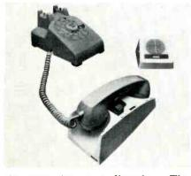
the user for easy listening. The speaker volume can be raised or lowered by turning the volume control. After a call is completed, the RCA TA100 reportedly shuts off automatically when the handset of the phone is lifted off the device and returned to its cradle.
