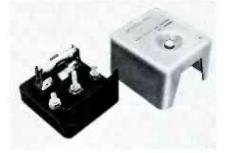
Manufactured by Telecommunications Industries Inc., the Model 300 TV and FM Receiver Protector is connected to the twin-lead antenna transmission line at the point where it enters a building or at the receiver itself. When an over-voltage occurs on the transmission line, a fusible spacer melts, placing a permanent short circuit across the line and grounding both sides of the line. The spacer is replaced to renew service.
