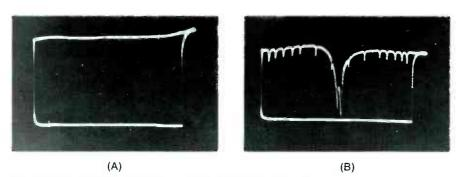
**Fig. 3** Two examples of normal sweep functions with satisfactory equipment. If you don't get a curve through the receiver, check the equipment operation this way: A) Sweep generators set for 3-MHz deviation with a center frequency of about 44 MHz. The output is almost perfectly flat. B) Sweep generator adjusted for video frequencies; output through absorption-marker box to video detector probe and scope.
