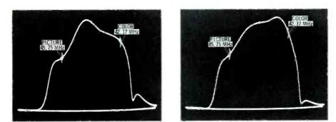
Fig. 11 Link alignment curves obtained when T204 is adjusted too far in either direction.
