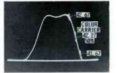
Fig. 14 Six markers, not just two, are required for accurate IF alignment. The three markers on the color carrier side are the most critical.
