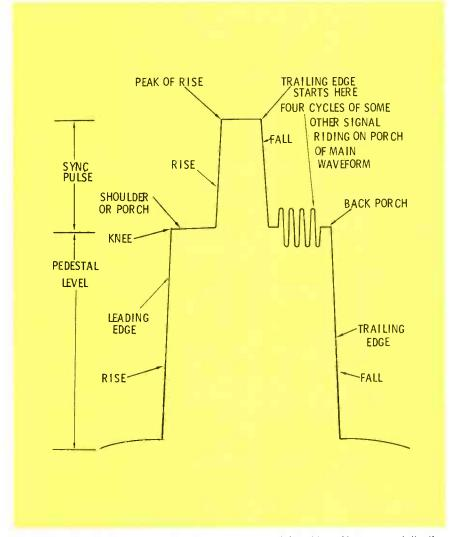
Fig. 2 Exaggerated version of horizontal sync and blanking. Note especially the leading edge; that's what triggers.
