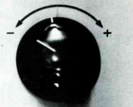
Fig. 1 STABILITY sets sensitivity of sweep oscillator; TRIGGER chooses point on slope of waveform where sweep fires.
