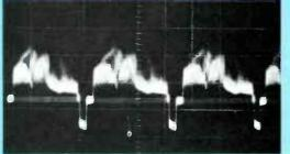
Fig. 4B, but locked in solidly. In A, the control is set just a little up from zero in the negative direction. In B, the trigger control has been advanced far negative. Much further and it would be beyond the waveform tip, and the screen would be blank.
