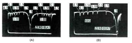
Fig. 16 A) Video sweep with absorption markers has a reversed curve on each side of zero beat. B) Adjust the sweep width and frequency to obtain a single curve.
