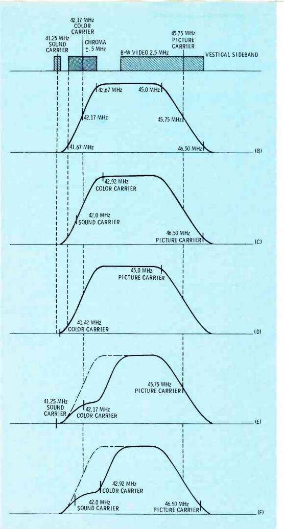
Fig. 2 The frequencies of the picture, sound and color carriers and their position on the IF curve are changed by the fine-tuning adjustment. The shape of the response curve and the frequency of the carriers determine the quality of both the b-w and color pictures.
