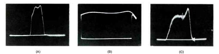
Fig. 9 Several curves produced by wrong equipment adjustments. A) Narrow curve caused by excessive (10 MHz) sweep width. B) Wide and incomplete curve caused by insufficient sweep width. C) Noisy and peaked curve with excessive gain caused by wrong AGC bias (between +65 and +70 volts).
