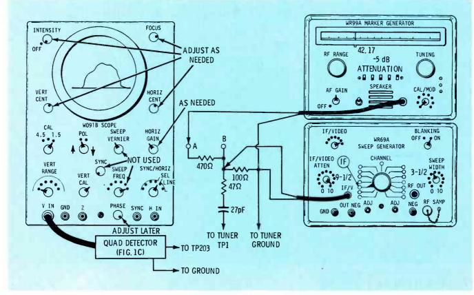
Fig. 4 Scope and generators preset for link alignment.
