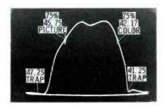
Fig. 7 The correct link curve with both color and picture carriers at 75%.
