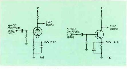
Fig. 2 Simplified sync separators. A) Vacuum tube circuit. B) Transistor circuit.
