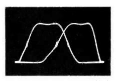
Fig. 8 With the sweep generator blanking turned off, two curves side by side indicate the scope phase control should be adjusted to bring them together.
