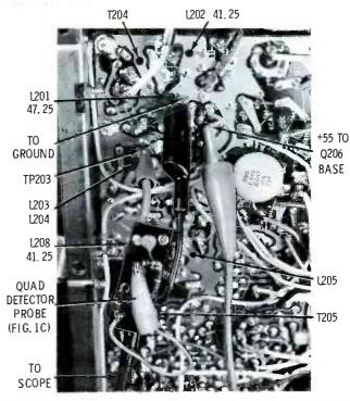
Fig. 6 Attach the "quad" detector probe to TP203 and ground, and connect the  $\pm$  55 volts from the external AGC bias control to the base of Q206.
