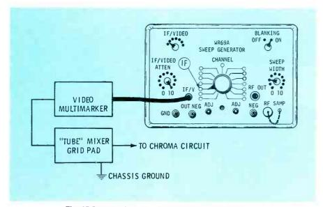
Fig. 15 Prepare the sweep generator as shown here.
