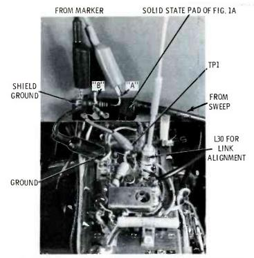
Fig. 5 Attach the sweep cable with the solid-state pad of Fig. 1A to TP1 on the tuner. Attach the marker cable to ground and point "A" on the solid-state pad.
