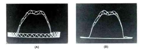
**Fig. 12** Adjust the 41.25-MHz and 47.25-MHz traps for minimum 600-Hz signal on the base line with the marker generator set for their respective frequencies. A) The trap is off frequency. B) The trap is adjusted correctly, and very little 600 Hz is seen on the base line.
