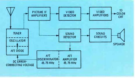
Fig. 1 AFT is a "closed loop" system for adjusting automatically the picture carrier to 45.75 MHz.
