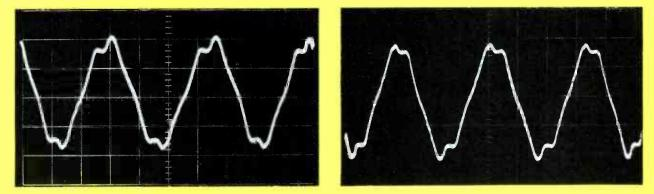
Fig. 3 Power-line sine waves. (A) is triggered near zero on negative side; (B) is triggered far negative from zero.
