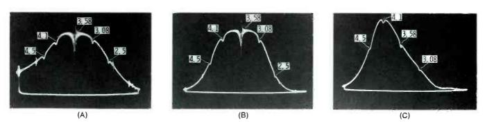
Fig. 17 Preset controls to obtain approximation of expected curves in chroma circuit. A) T705 only. B) T705 and T701, C) T705, T701 and L701.
