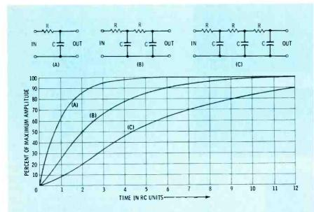
Fig. 16 Universal time-constant chart for one-section, two-section, and three-section integrator circuits.
