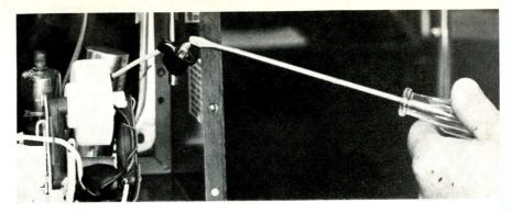
Fig. 4 Removing the rectifier plate cap and again drawing an arc to determine whether the trouble is before or after the high-voltage rectifier tube. (Although the screwdriver blade here appears to be touching the metal cabinet, it actually is more than an inch away.)
