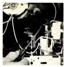
Fig. 2 If a suitable arc can be drawn from the plate cap of the high-voltage rectifier, the horizontal oscillator and output tubes, flyback transformer, damper circuit and B+ are probably okay
