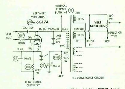
Fig. 8 C4 and R108 commonly cause insufficient height in CTC16 chassis.
