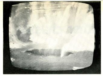
Interference caused by poor ground connection between chassis and CRT of portable color chassis.
