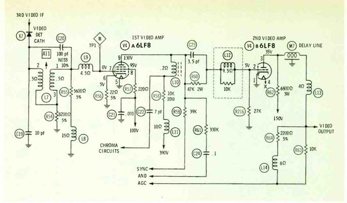
Fig. 4 Check L8, L13 and L14 and their associated solder connections when the trouble symptom is a smeared or blurred picture.
