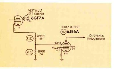
Fig. 9 A change in the values of resistors R127 and R128 cause vertical height problems.
