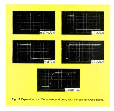
18 have a basic characteristic called "rise time" (or fall time) that can be measured with a lab-type scope. This category of waveform analysis is not pracical with a simple servicetype scope.
