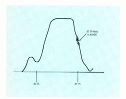
Fig. 4. The 45.75-MHz marker falls right above the 45.75-MHz position on the base line of this hand-drawn curve. You can imagine the same for markers put on response curve by a generator.
