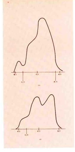
Fig. 3. Oddly shaped response curves indicate trouble in tuned circuits of IF strip. (A) Coil usually peaked at 42.5 MHz has shifted to about 44 MHz, and adds to response of coil already peaked at 44.5, creating exaggerated peak. (B) Trap normally at 41.25 MHz has shifted to about 43.5 MHz; eliminates the dip needed at 41.25 MHz, and introduces unwanted dip slightly above 43.0 MHz.
