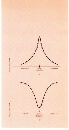
Fig. 1 Graph of meter readings as tuned circuit is adjusted to, through and past resonance with applied signal frequency. Curve at B is tuning response of a trap.
