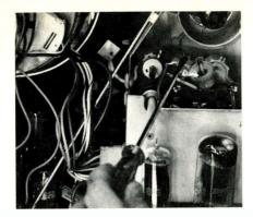
Fig. 3 Checking the arc with the highvoltage rectifier plate cap of a color TV removed can cause damage if the arc is sustained more than three or four seconds. Note in this photo that the high-voltage pulse of this color set is not only arcing to the screwdriver but also from the screwdriver to a terminal on the flyback. If the screwdriver is removed, the arc will still flash over to terminals or chassis points over an inch away, unless the sweep circuit is defective.
