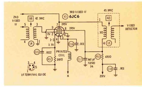
Fig. 3 When the 3rd video IF amplifier shorts, it also usually destroys the plate-load resistor, R53.
