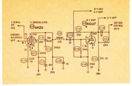
Fig. 12 A leaky coupling capacitor (C133) between demodulator and color difference amplifier and over-heated plate-load resistors (R192) can cause a missing color and intermittent color, respectively.
