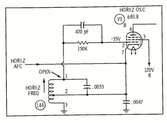
was slightly above normal. The voltage at the cathode of this stage was 200 volts instead of the normal .23 volt.
