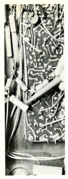
Fig. 7 Vertical feedback capacitor C71, pointed out here, has a long history of failure in the CTC16 chassis. When leaky or shorted, this capacitor reduces the vertical sweep to a horizontal white line.
