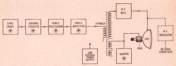
Fig. 1 Block diagram of the TV stages in which common defects can reduce or completely kill the high voltage.
