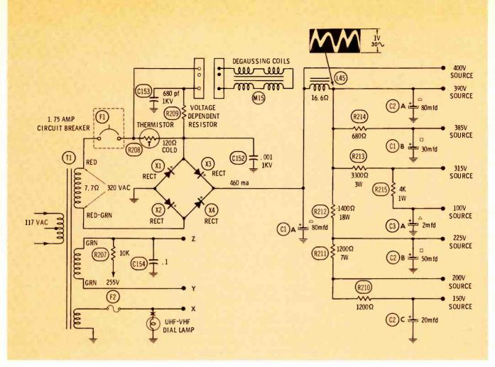
Fig. 2 Shorted or open diodes and a defective C1A are prime causes of hum in the sound and raster of the RCA CTC16 chassis.
