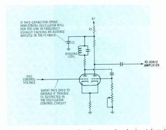
Fig. 6 Simplified schematic diagram of a horizontal multivibrator circuit which employs a decoupling network, R1 and C1, in the plate circuit. If C1 opens, the oscillator frequency will be reduced, and an audible whistle in the flyback probably will be heard.
