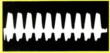
Fig. 23 Bandpass-amplifier output waveform has sloping sides and rounded corners.
