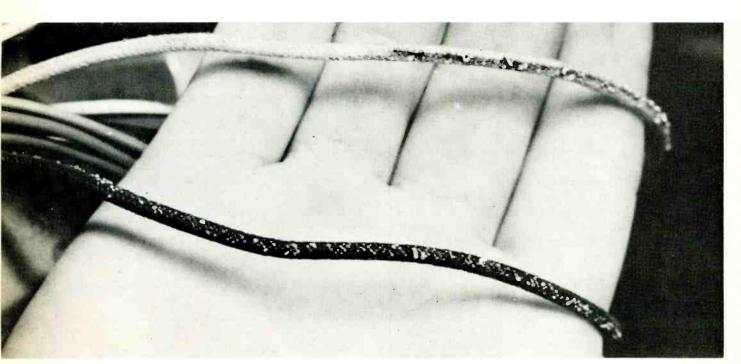
Fig. 1 This photo shows the results of a stuck circuit breaker. Notice the beads of solder on these AC leads, which were connected to the on/off switch. The wire was coated with solder, and when an excessive amount of current passed through them, the solder popped out through the insulation—a visual indication of the source of the overload. In this case, the power transformer was also "cooked."
