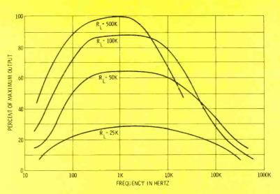
Fig. 22 Frequency response versus plate-load resistance for an RC-coupled stage.
