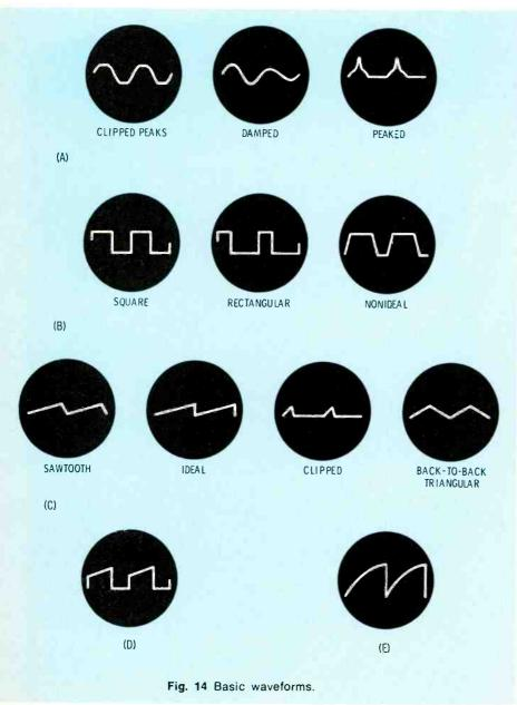
as shown in Fig. 9B. These sine waves are harmonically related, and have the relative amplitudes shown in Fig. 10. These facts are of considerable importance in practical troubleshooting procedures, because analysis of distorted pulse or square waveforms will provide clues concerning circuit defects. For example, some of the most basic distortions and their causes are shown in Fig.
