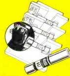
BUSS KAZ Actuator 13/32 x 2 in. Sig-Use to call attention to the opening of a fuse of 50 amp or larger. Can be mounted "piggy-back" on large fuse or in special block with micro-switch. Ask for Bulletin KAFS.
