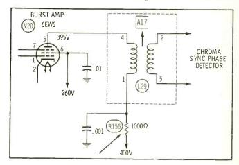
that adjustment of L29 had little or no effect. A check with the scope revealed that there was burst present on the grid of the burst amplifier, but none on the plate. Using a VTVM, I discovered that the voltage
