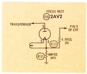
Fig. 11 An increase in the value of R131 or R133 will produce poor focus.
