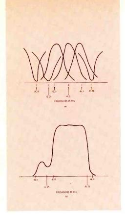
Fig. 2. Group of individual voltage-response curves (A), when combined, make up overall response curve (B). Shows voltage indications at every frequency within the band of signals to which a television IF section responds.
