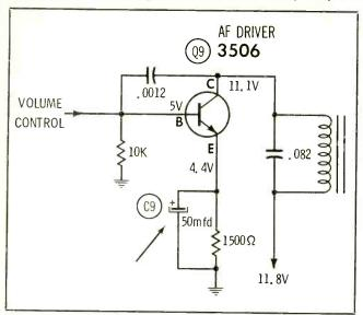
audio driver stage was below normal. Component checks in this stage isolated the trouble to an open bypass capacitor (C9) in the emitter circuit of the audio driver. Total troubleshooting time: 15 minutes.
