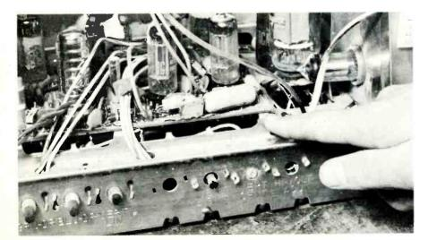
Fig. 13 Poor ground connections on chroma and video circuit boards can cause hard-to-solve trouble symptoms.
