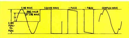
Fig. 2 Five waveforms that have the same peak-to-peak voltage.
