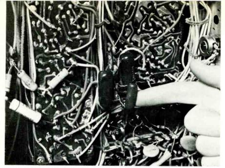
Fig. 10 C143, a .056-mfd capacitor in the horizontal efficiency coil circuit, is a prime source of overload in the high-voltage section.
