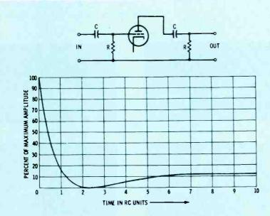
Fig. 17 Universal time-constant chart for RC-coupled amplifier with two RC sections.
