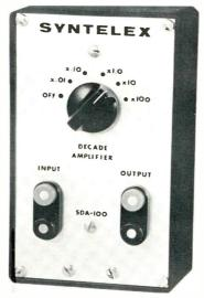
as having these specifications: voltage gain (selected by switch) of X100, X10, X1, X.1, X.01 with a frequency response from 10 Hz to 1MHz; input impedance of 1.11 megohms; a maximum input level of 100 volts rms; output impedance of 100 ohms; a maximum output level of 10 volts peak-to-peak; and an equivalent input noise figure of 50 microvolts.
