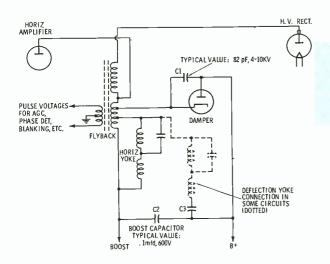
Fig. 5 Simplified schematic diagram of a common flyback circuit.
