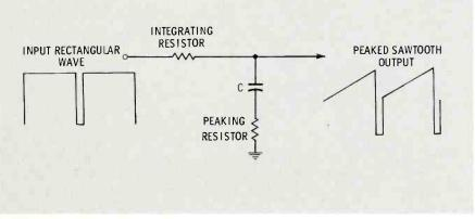
Fig. 10 Resistance-type peaking circuit.
