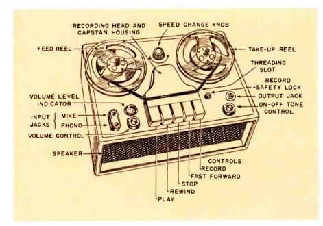
Fig. 1 Typical two-speed recorder with principal features indicated.
