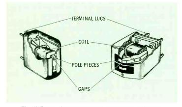
Fig. 10 Detail of typical erase (A) and record (B) heads.
