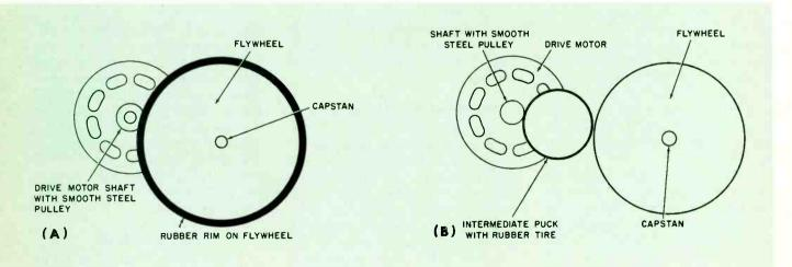
Fig. 16 Two methods of capstan drive. (A) Rim drive to flywheel. (B) Intermediate-puck drive.
