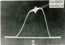
Fig. 2 Photos illustrating the advantage of using a low-pass filter between the probe and the input of the scope. (Probes shown in Fig. 1 have a builtin low-pass filter.) A.) Curve produced using a probe without a low-pass filter —the marker covers the whole curve. B.) Curve produced using a low-pass filter in the probe—marker is much sharper.
