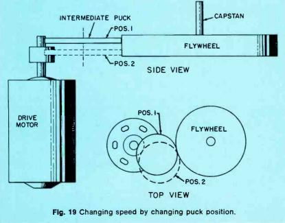
worn, glazed or dented. Defective tires must be replaced. Drive trouble can also be caused by a film of oil on the idler tire. It may be possible to restore normal operation by thorough cleaning with carbon tet or an equivalent. Since carbon tet has poisonous fumes, equivalent solvents are preferable.
