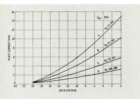
Fig. 3 Dynamic transfer characteristics for different loads.
