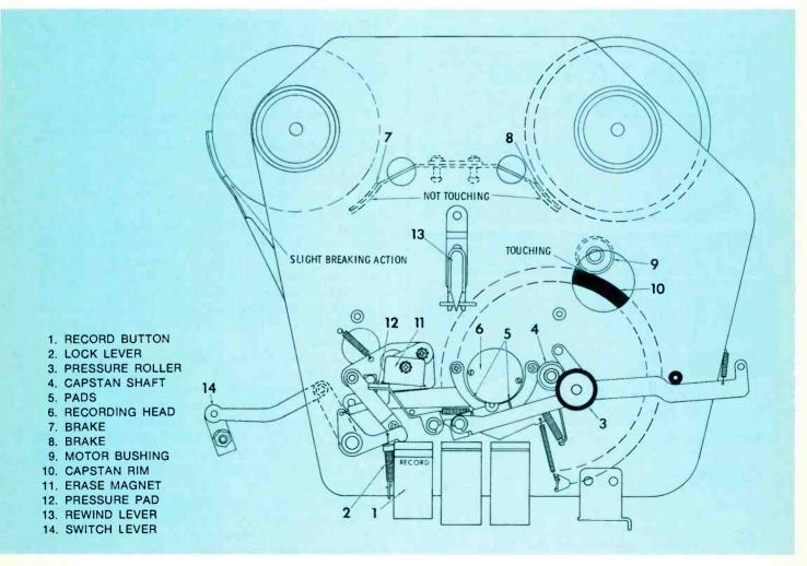
Fig. 21 Top view of tape transport mechanism in "Record" position (33/4 in./sec.).
