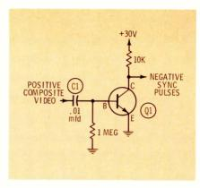
Fig. 5 A simplified sync separator.
