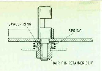
Fig. 8 A tape guide with a stop control pin assembly.
