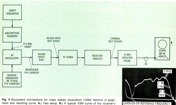
ment and resulting curve. **A**.) Test setup. **B**.) A typical VSM curve of the receiver's response from tuner to video detector output. (Do **not** align the IF's using this curve.)
