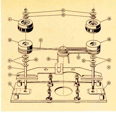
Fig. 14 Typical belt-drive clutch assembly.
