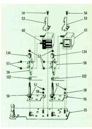
Fig. 9 Exploded view of a typical head assembly.
