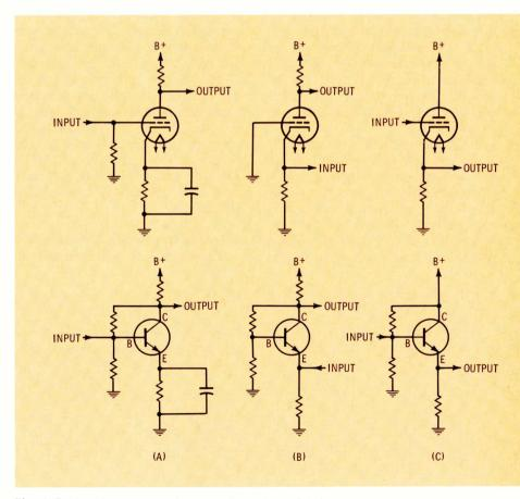
Fig. 1 Basic tube and transistor configurations. A.) Common cathode and common emitter. B.) Grounded grid and common base. C.) Cathode follower and emitter follower.
