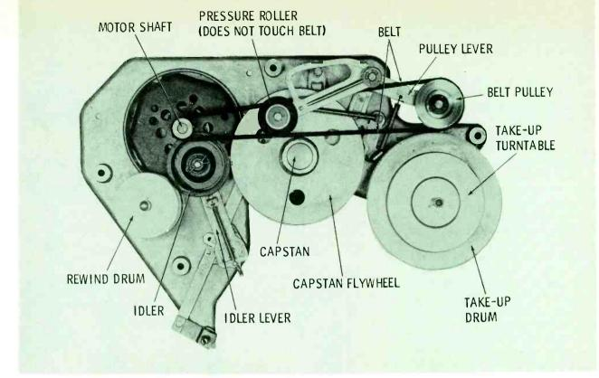
Fig. 15 Transport mechanism of a conventional tape recorder.
