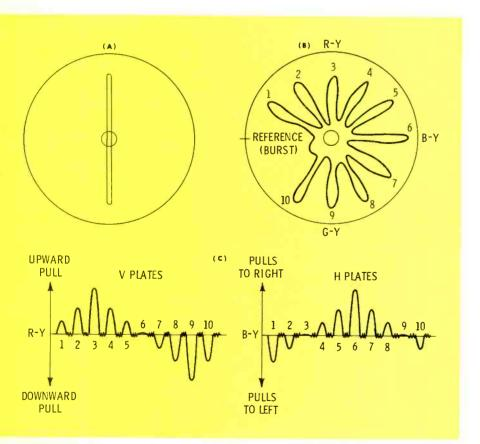
Fig. 2. How vectorgram is formed on vectorscope CRT. (A) R-Y connected to vertical deflection plates. (B) B-Y connected to horizontal deflection plates matrixes with R-Y to form "starburst" or "daisy" display. (C) The two signals as you'd see them on an ordinary wideband servicing scope; they combine in vectorscope to form the display.
