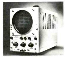
is designed for educational, laboratory and servicing applications. It is capable of accurate phase comparison and measurement involving Lissajou functions and differential
