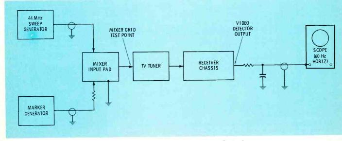
Fig. 3 Equipment connections for IF-sweep curve alignment.
