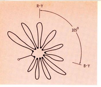
Fig. 5 This leaning, elliptical vectorgram is the pattern formed from 105-degree demodulator.
