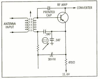
a defect in it was not directly responsible for the varying collector voltage. I then measured the emitter voltage; it was varying from 11 volts to less than 7 volts. I checked the voltage across the emitter resistor; it was varying from approximately .4 volt to over 5 volts. Again, the noise disappeared and the radio returned to normal operation.
