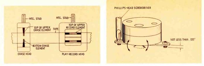
Fig. 11 Proper head height location.
