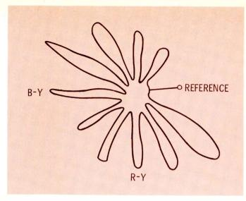
Fig. 6 When cathodes of CRT are driven, phase of the vectorgram is rotated 180 degrees.
