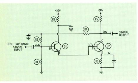
Fig. 4 Two-stage amplifier with feed-back bias stabilization.
