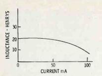
Fig. 11(a) Magnetizing inductance of vertical-output transformer versus current.
