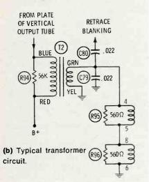
stage undercompensates the exponential curvature of the drive waveform. From previous discussion, it follows that the bottom of the picture will be compressed by this circuit defect.
