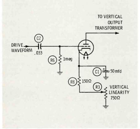
Fig. 12 Capacitors C1 and C2 affect vertical linearity.
