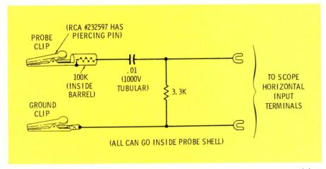
Fig. 3 Homemade probe for adapting any servicing scope to vectorscope servicing.
