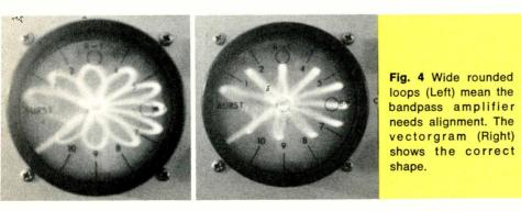
adjust the vertical and horizontal gain controls to make the vectorgram round. You may have to juggle position controls to center the display.
