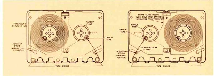
Fig. 13 Design of conventional tape cartridge.
