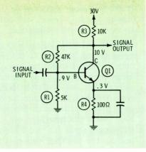
Fig. 3 Example of a transistorized amplifier.
