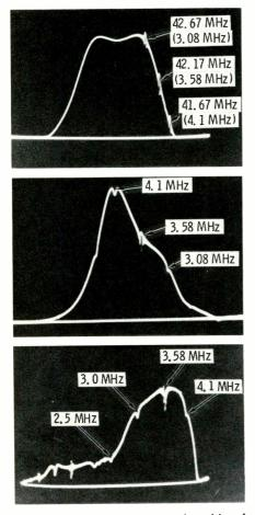
Fig. 5 Adding the color-carrier side of the IF curve (A) to the overall chroma IF curve (B) produces the VSM curve (C) at the chroma demodulators.
