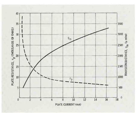
Fig. 9 Triode transconductance and plate resistance versus plate current.
