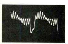
Fig. 1 Display on ordinary service scope connected to red grid of CRT. Phase is adjusted till sixth bar is right on base line.
