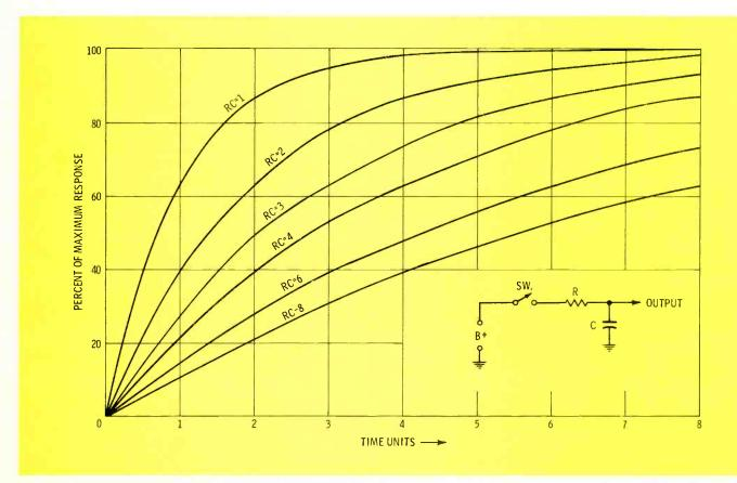
Fig. 2 Integrator waveforms for various time constants.
