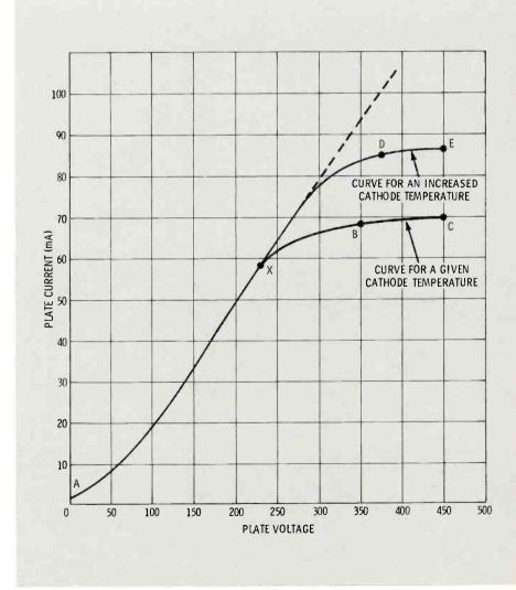
Fig. 6 Plate-current plate-voltage characteristic curves.
