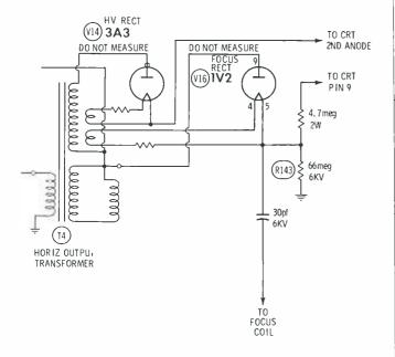
We have also experienced streaking flashes in the picture, similar to high-voltage arc, and traced it to the focus load. Evidently this resistor can cause a multitude of symptoms, depending on the type of resistor defect, and the particular chassis involved.
