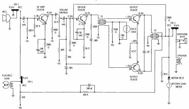
Fig. 2. Schematic diagram of typical low-priced tape recorder.
