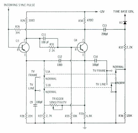
Fig. 4. Partial schematic of trigger stages.
