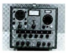
Included is a "dial-in" feature that allows users to "dial-in" any frequency in the FM communications spectrum. Once the frequency is selected, frequency error and FM deviation can be read simultaneously. The whole process takes less than 10 seconds. Frequency accuracy is better than .000075% long term.
