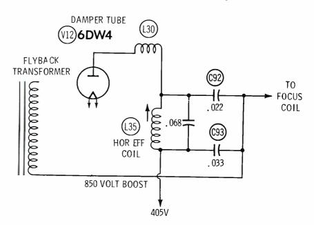
Fig. 8. Shorted C93, resulted in reduction of high voltage.
