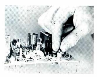
The unique "plugability" concept is carried throughout the entirely new Sylvania chassis. Called the "Gibraltar," the chassis has a plug-in tuner cluster, plug-in deflection yoke, plug-in convergence section, plug-in automatic degaussing section, plug-in speakers, and a plug-in remote control unit.
