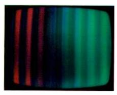
B-W picture OK. Blue missing from color programsknown blue portions of picture now green-normal tint control action missing—flesh tones not "purplish" at one extreme. Generator pattern confirms symptom red and green OK but blue poor.
