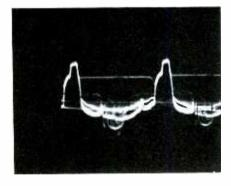
(B) Sync separator waveform.
