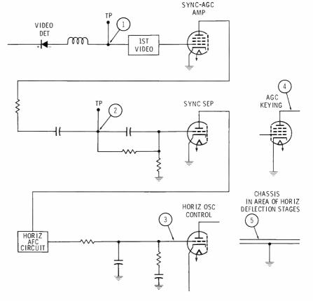
Fig. 1. Radiation pulse was viewed in several circuits and on the chassis.
