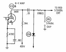
Fig. 4. Shorted silicon diode X14 caused red screen.
