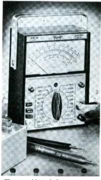
The portable unit has an accuracy of  $\pm 2\%$  of full scale on DC and  $\pm 3\%$  for AC, with a frequency response on the AC from 50 Hz to 50 kHz. Another interesting feature is the low-power ohms measurement circuit for integrated circuit (IC) applications.
