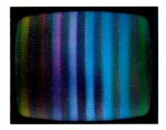
Reds seem much weaker than greens and blues on color programs. Level and tint controls operate but impossible to get proper flesh tones. B&W background is reddish—screen control adjustment corrects—but then red is lost completely on color programs.
