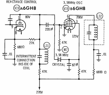
Fig. 5. Deflective coil caused intermittent color.
