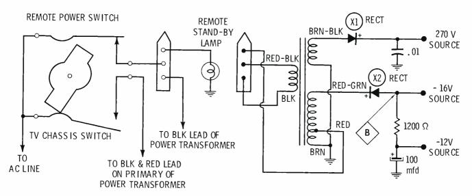
Fig. 8. Power supply provides low voltage for transistors and high voltage for transducer.
