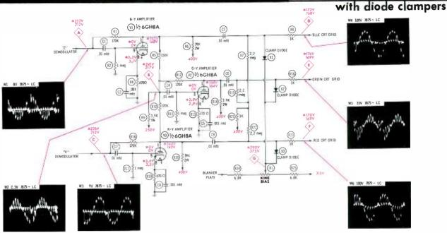
DC VOLTAGES taken with VTVM—no color signal input. \*Indicates voltage taken with color-bar input—see "Operating Variations".
