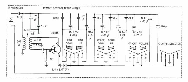
Fig. 3. Transmitter has eight output frequencies.
