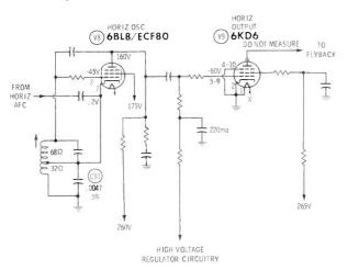
The normal cathode current of the horizontal-output tube is 220 ma. Assuming a 150% overload is sufficient to destroy the tube, this would increase the total current through the circuit breaker from 460 ma. to 570 ma., an increase of less than 30%. Circuit breakers normally are designed to open if the current exceeds 150% of the design value. For further information on the subject, read "The Circuit Breaker is Trying to Tell You Something", PF REPORTER, February, 1968.
