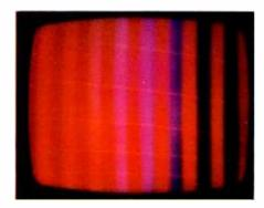
Black-and-white picture with red background obtained by adjusting brightness and contrast controls. Red is predominate color in color programs. Tint control has little effect since red is only color. Color level controls amount of red—other colors hardly noticeable.
