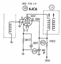
Fig. 1. Resistor R52 overheated.
