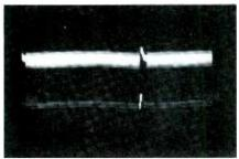
Fig. 3. Trace shows good vertical lock.
