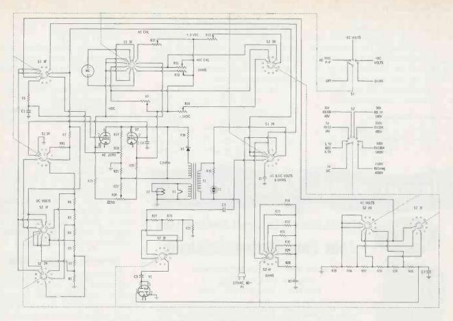
Fig. 6. Complete schematic diagram of vacuum-tube voltmeter.
