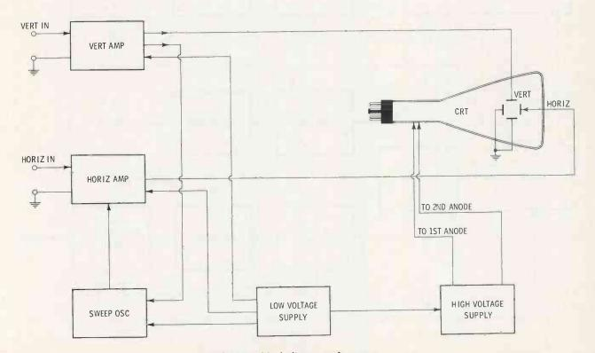
Fig. 1. Basic block diagram of a scope.
