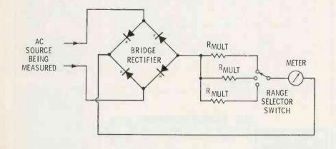
Fig. 5. Bridge-type rectifier circuit for measuring AC voltage.
