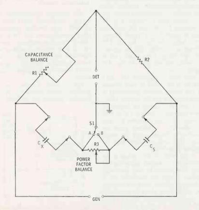
Fig. 14. Universal bridge employing power factor balance control.
