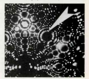
In the photo above, the arrow points to a single atom of tungsten. The new microscope, called the atomprobe, field-ion microscope, is currently being developed by Professor Erwin Mueller at the Pennsylvania State University.
