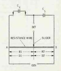
Fig. 10. Basic slide-wire bridge used for measuring capacitance.
