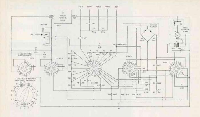
Fig. 4. Complete schematic diagram of typical volt-ohm-milliammeter.
