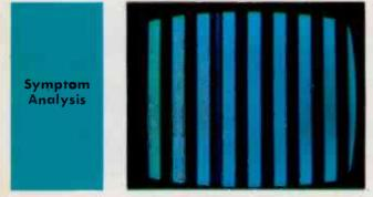
Almost normal color with chroma gain at maximum on local station; little or no color on fringe station. Generator signal color bars in correct order but weak. Tint control operates when color present. B-W picture normal. Symptom indicates chroma signal loss.
