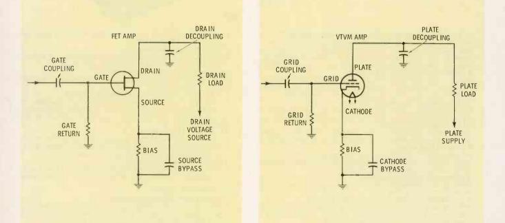
Fig. 9. Comparison of amplifiers employing field-effect transistor and vacuum tube.
