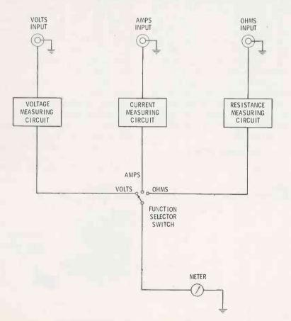
Fig. 3. Block diagram of VOM emphasizes isolation between functions.
