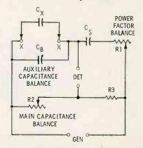
Fig. 17. Substitution method permits measurement of low values. calibrated variable capacitor,  $C_{\rm B}$ , connected to the unknown terminals, X-X. This capacitor is usually a 100or 1100-pf air type having a dial reading directly in picofarads. In all other respects, this bridge is identical to the one shown in Fig. 15.
