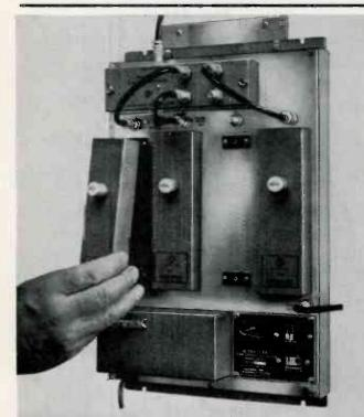
82-Channel Ultra-Plex System using lo band plug-in VHF amplifier ...hi band plug-in VHF amplifier... and broad bard UHF amplifier.
