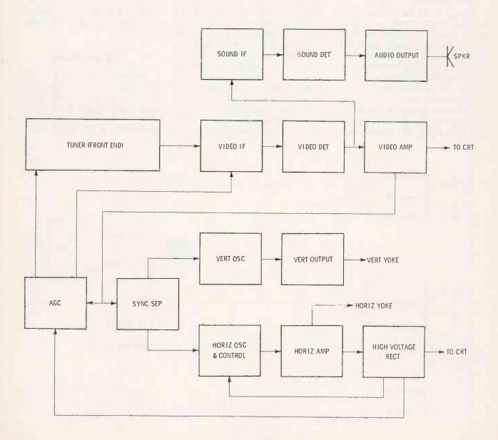
Fig. 2. Basic block diagram of a black-and-white receiver.
