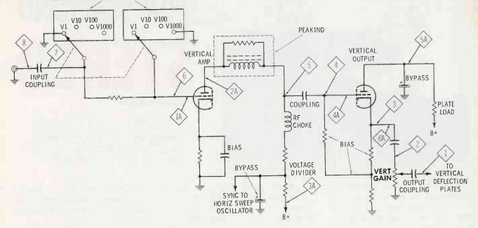
Fig. 3. Typical simplified vertical amplifier circuit.
