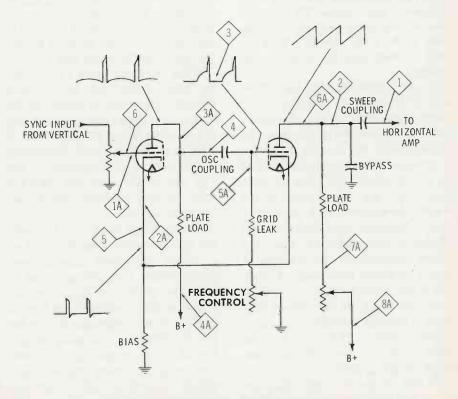
Fig. 4. Typical sweep oscillator circuit.
