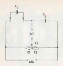
Fig. 11. Slide-wire capacitance bridge employing wirewound potentiometer.
