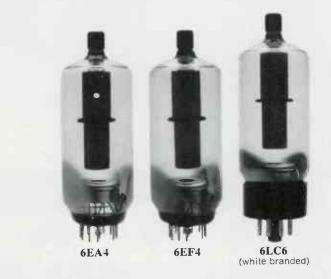
In early 1967, General Electric started a modification program to eliminate the possibility of soft downward x-radiation emission from some of its large screen color television receivers. This modification program, which involved replacement of the obsolete regulator tubes pictured above, is now complete except for a very few receivers which have not yet been located.
