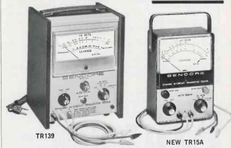
Locate defective transistors in circuit in seconds with a true AC signal gain test (BETA) . . . without disconnecting a single lead . . . what a time saver. Also measure AC beta and Icbo leakage out of circuit for complete analysis of the transistor. It's easy, fast and accurate. Also checks diodes and rectifiers in and out of circuit.
