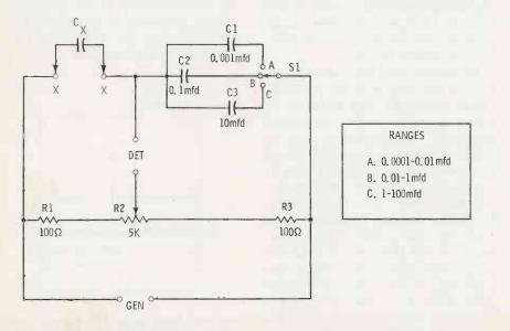
Fig. 12. Practical slide-wire bridge for measuring capacitance.
