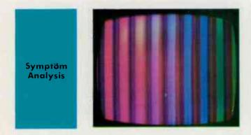
Color programs show excesive red—also, areas that should be white are red. Near normal color picture obtained by misadjusting tint and color controls. Screen is tinted red with color signal; but with chroma gain control at minimum b-w picture has proper gray scale.
