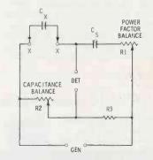
Fig. 15. Capacitance comparison bridge is similar to Wheatstone design.
