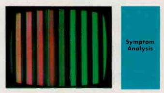
Loss of blue evident on station color programs—whites have yellow tint, other colors using blue are wrong. Tint and chroma gain controls operate. Bar pattern shows only green and red—blue missing and background yellow with chroma gain at minimum. B-W normal.
