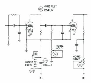
Thanks to you, too. Mr. Daly, for confirming our diagnosis. The original problem was an RC-101 TV receiver (PHOTOFACT 142-10) that would drop out of sync during warmup. Our advice: "The trouble is probably caused by a thermal drift of one of the frequency determining components in the horizontal oscillator.
