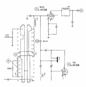
As an alternative to the injection point "B", you may clip pin 9 from the 6CQ8, and inject the signal at the test point (it's in a hole in the chassis), or through an ungrounded tube shield. Clipping pin 9 disables the oscillator. A slightly weak or used 6EA8 or 6U8 with pin 9 clipped will work equally well in this case, since the operating frequency and amplification are of slight importance. The main thing is to couple a signal to the plate.
