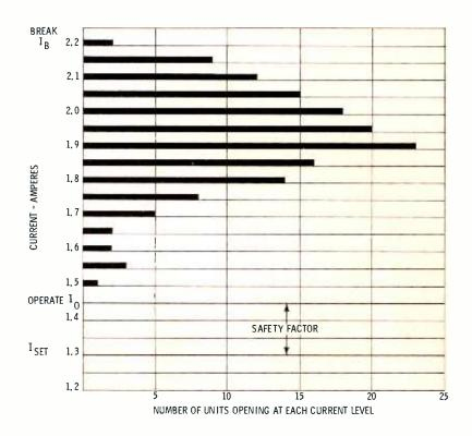
Fig. 2. An analysis of the actual operating range of a group of circuit breakers.
