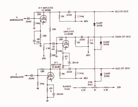
Fig. 10. CRT grid clampers of RCA Chassis CTC27.
