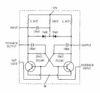
Fig. 4. Typical divider stage.
