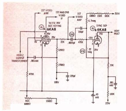
Fig. 3. Heat sensitive capacitor caused intermittent defect.
