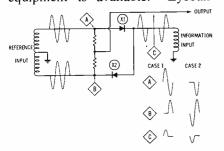
Fig. 1. Simplified phase-sensitive detector using diodes.
