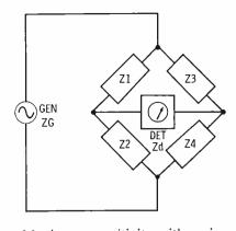
Maximum sensitivity with a given fixed-output generator and fixedsensitivity detector is obtained when  $R_1 = R_2 = R_3 = R_4 = R_g = R_p$  in the DC bridge, and when  $Z_1 = Z_2 =$  $Z_3 = Z_4 = Z_G = Z_p$  in the AC bridge. (The symbol  $R_G$  or  $Z_G$  is the generator output resistance or impedance;  $R_p$  or  $Z_p$  is the detector input resistance or impedance.)
