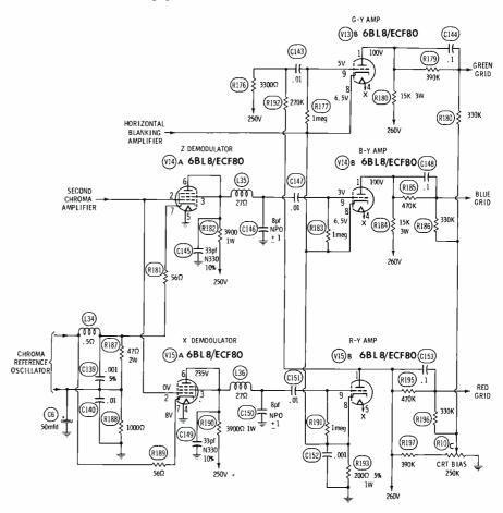
Fig. 4. Chroma demodulators and color-difference amplifiers of the Philco 17QT85A chassis.
