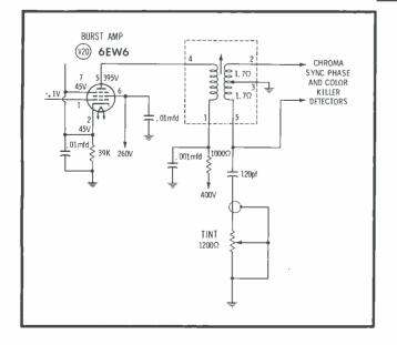
Mfr: General Electric Chassis No: CA Card No: GE CA-6 Section Affected: Color pix. Symptom: Tint control has no effect on hue. Cause: Shorted cable in tint control circuit.
