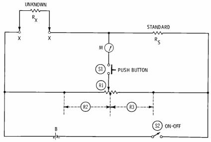
Fig. 5. Slide-wire resistance bridge employing a potentiometer.
