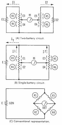
Fig. 2. Evolution of the bridge from two-battery circuit to present design.
