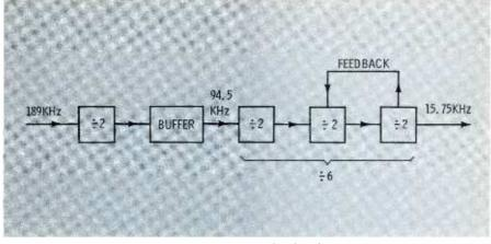
Fig. 5. The horizontal divider chain.
