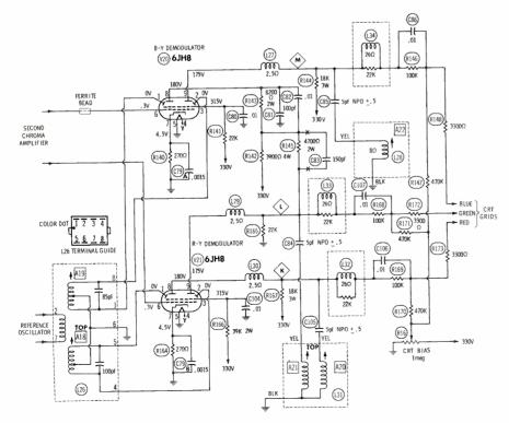
Fig. 7. Sheet-beam demodulator of Zenith Chassis 24MC32.
