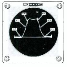
SIX MARKERS SIMULTANEOUSLY. The scope trace above shows how six markers can appear at the same time. Note the trap markers, 6 dB points, and picture and sound carriers... all on one trace with the IG-14.
