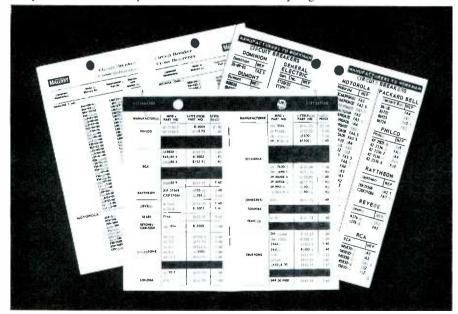
Fig. 3. A circuit breaker cross-reference chart aids replacement.
