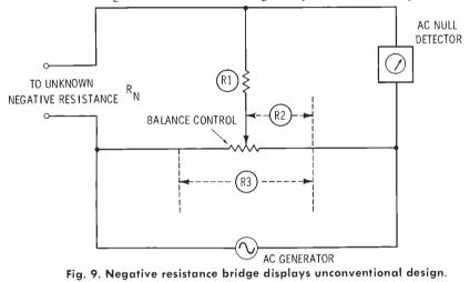
ing  $R_x$  under actual working conditions and to provide an off-balance output voltage high enough to ensure accurate null adjustment.
