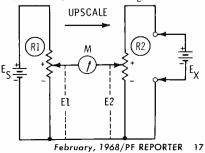
ogy, the power source (such as the battery in Fig. 2C) is termed the *generator*, and the null indicator (such as the center-zero galvanometer in Fig. 2C) is the *detector*.
