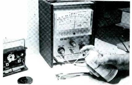
Fig. 1. Set up for checking intermittent transistor.
