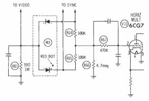
Unfortunately, there was an error in the PHOTOFACT. As can be seen the actual resistance will be 470K ohms plus the resistance made up of R66 in parallel with R64, R65. M3, and R81. Since the resistance of M3 can vary widely, depending on the ohmmeter used, the reading could be anything from about 600K ohms to several megohms. The 1.3 megohms you measure sounds reasonable.
