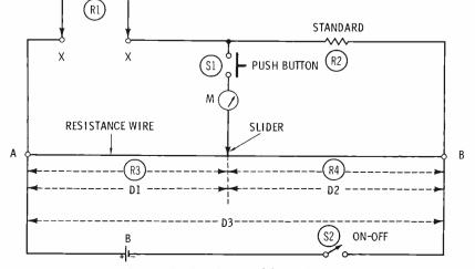
Fig. 4. Basic slide-wire bridge designed for resistance measurements.
