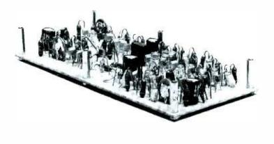
Fig. 3. Sync and horizontal board.
