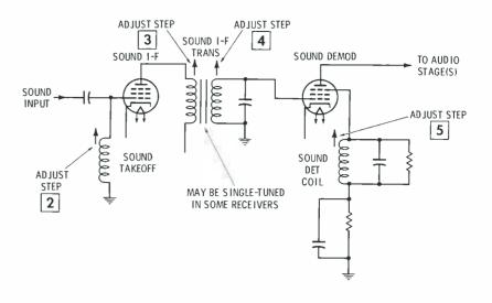
Fig. 1. Typical sound system in current color TV receivers.
