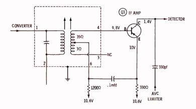
Fig. 4. Defective IF amplifier stage in Ford Model 6TBF car radio.
