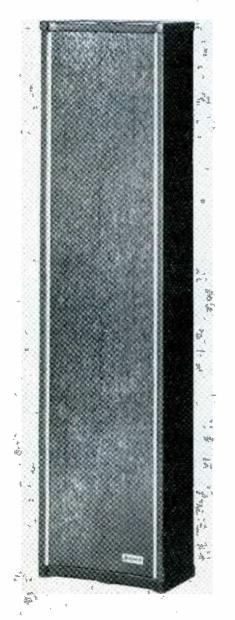
Fig. 8. The Jensen HFC-84 is a 100watt column speaker with a 30° vertical angle of sound radiation. 50 to 15,000 Hz, and the speaker coverage angles are  $100^{\circ}$  horizontally, but only  $30^{\circ}$  in the vertical plane. The input impedance is 8 ohms, but a well in the top of the enclosure accommodates a matching transformer, if one is required. Screw terminals within the well permit installing the transformer without solder.
