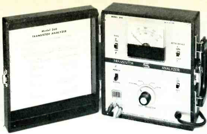
Fig. 3. New transistor tester has no Beta Cal control.
