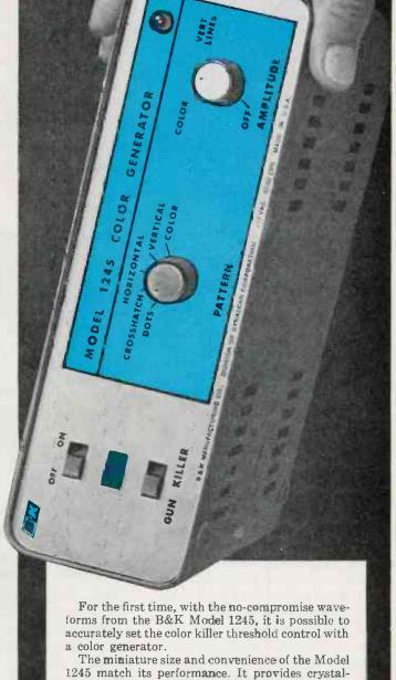
controlled keyed rainbow color bar display, and dot, crosshatch, horizontal line and vertical line
