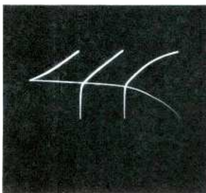
Fig. 10. Effects of poor horizontal linearity on deflection waveform.
