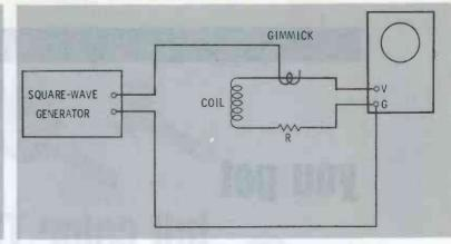
Fig. 3. Test setup with arbitrary resistance connected in series with coil.
