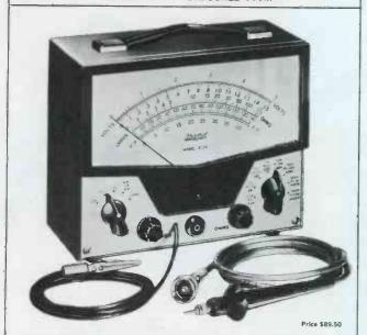
Advanced UNI-SCALE design reduces reading errors and simplines usage because nurr basic scales is reduced to TWO for all AC and DC ranges. 60% less DC, 40% less AC loading.
