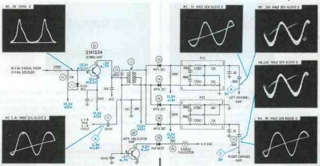
DC VOLTAGES taken with VTVM; receiver off station. \*Indicates voltage taken with signal from stereo generator present — see "Operating Variations." WAVEFORMS taken with wideband scope, receiver controls set to produce normal stereo FM sound. D (direct) probe used for testing where indicated.
