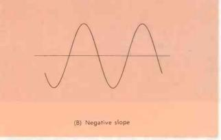
Fig. 9. Waveforms friggered on opposite slopes.
