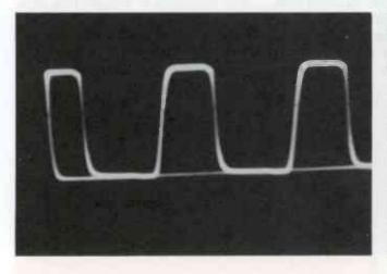
Fig. 4. Semi-square wave on free-running oscilloscope.
