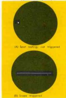
Fig. 2. Trigger control of CRT beam.
