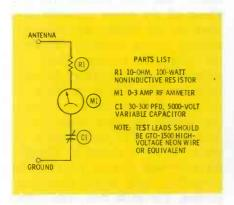
Fig. 1. Circuit diagram of dummy
