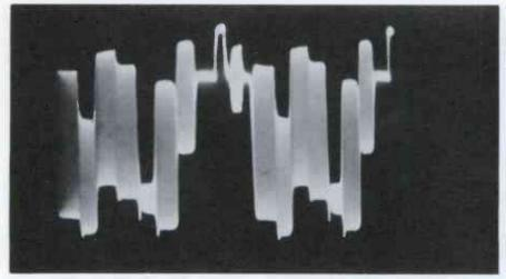
Fig. 13. Composite color waveform.
