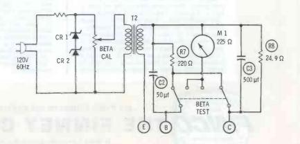
Fig. 3. Simplified schematic of the beta tester.
