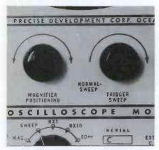
Fig. 1. Trigger and magnifier controls on triggered sweep scope.
