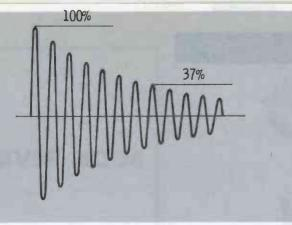
Fig. 2. Damped sine wave with 7 cycles between amplitude level of 100% and 37%.
