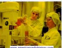
Screen Test! 330,000 dots in each color, must be no more or less than .018 of an inch in diameter. If not, panel is washed clean and a fresh start made.
