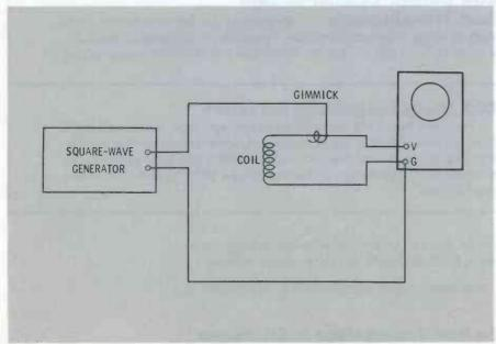
Fig. 1. Equipment setup to measure Q.
