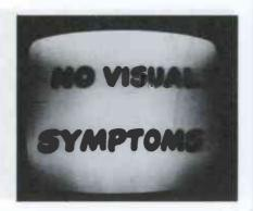
Left channel weak on stereo FM signal compared to right channel and has excessive noise (popping, cracking, etc.) and background "rush" noise. Separation poor. Monaural FM, AM, and stereo phono functions seem normal. Trouble suspected in stereo FM circuitry.
