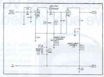
oscillator components that can also cause this symptom, it is impractical to attempt substitution. Instead, locate the faulty component with one of the freeze-sprays currently on the market. First, while the set is still cold, perform a quick horizontal alignment. Then when the set heats up and drops out of sync, spray the suspected components one-by-one until the set falls back into sync.
