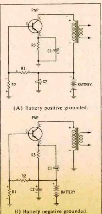
Fig. 3. Common-emitter amplifier using a PNP transistor.
