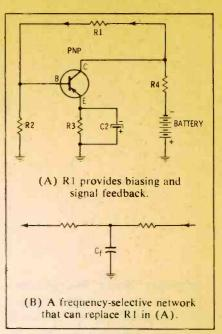
Fig. 4. Bias stabilization and feedback.
