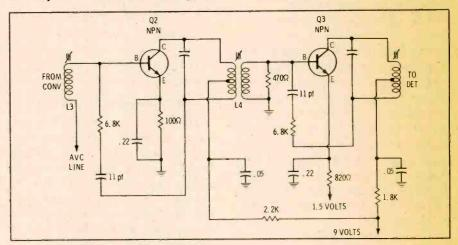
Fig. 10. An IF amplifier with single-tuned transformer.
