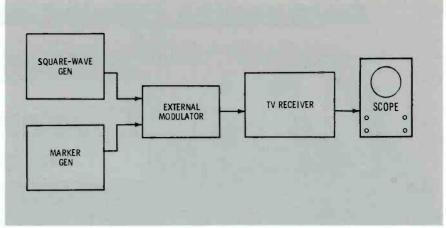
Fig. 4. Plan of test setup with an external modulator.
