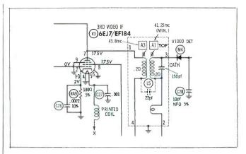
The beat pattern you are experiencing has also occurred in earlier RCA chassis and is a result of the 4th harmonic of the picture IF carrier, generated in the picture-detector circuit, being picked up by the 300-ohm lead associated with the UHF/VHF switch. The frequency of the interference is approximately 183 mHz, depending on the position of the fine-tuning control.
