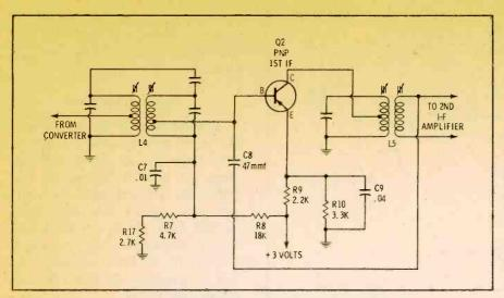
Fig. 11. An IF amplifier with double-tuned transformer.
