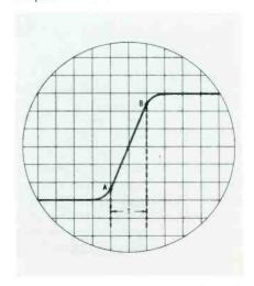
Fig. 9. Measure rise time from A to B.
