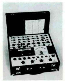
Fig. 1. High speed tube tester.
