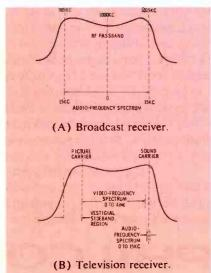
Fig. 1. Frequencies in the RF bandpass.
