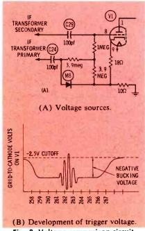
Fig. 3. Voltage-comparison circuit.
