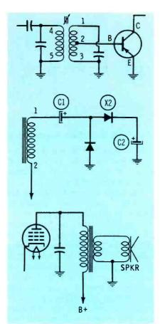
Fig. 8. A few of the many external circuits that affect transformer checks.
