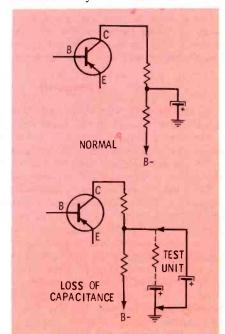
Fig. 4. Loss of capacitance has effect of resistor in series with electrolytic.
