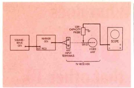
Fig. 10. Complete test setup for receiver check.
