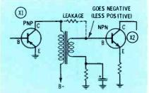
Fig. 9. Leakage has effect similar to leaky coupling capacitors.
