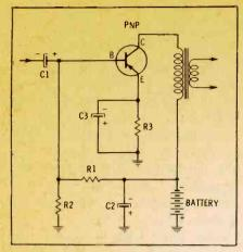
Fig. 5. Common R-C coupled circuit.
