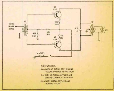
Fig. 16. A push-pull output stage with current drains.
