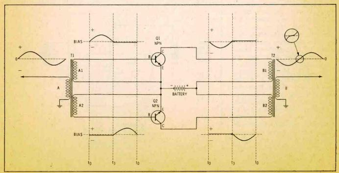
Fig. 14. A class-B output stage with current waveforms. (Waveforms are not drawn to scale.)
