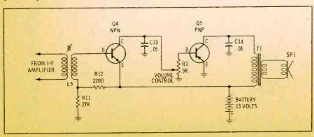
Fig. 9. A DC coupled amplifier employed in a receiver.
