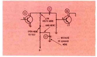
Fig. 7. If voltage becomes normal, C2 is bad. If not, trouble is in X1 or C1.
