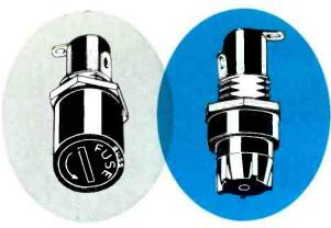
Screw type slotted knob that is recessed in holder body and requires use of screwdriver to remove or insert it. Screw type knob designed for easy gripping, even with gloves. Has a "break-away" test prod hole in knob.
