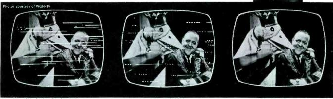
Unshielded twin-lead Severe picture disturbance due to ignition noise.
