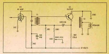
Fig. 7. A vacuum tube driving a transistor.
