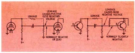
Fig. 5. Leakage in coupling capacitor affects bias on next stage.
