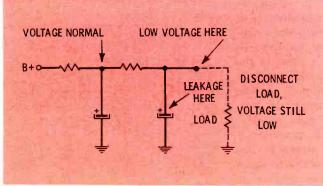
Fig. 6. Basic principle of finding short involves unsoldering loads.
