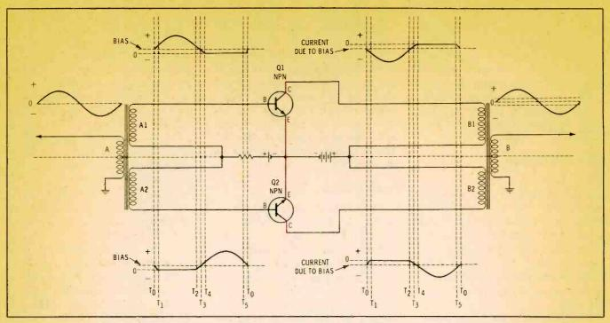
Fig. 15. A class-AB output stage with current waveforms. (Waveforms are not drawn to scale.)
