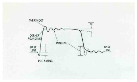
Fig. 7. Results of improper frequency.
