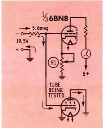
Fig. 2. Simplified schematic shows how grid-emission test is accomplished.
