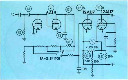
Fig. 4. VTM circuit shown in AC function (much simplified).
