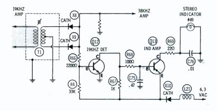
Fig. 1 Schematic Magnavox R204 EP chassis.
