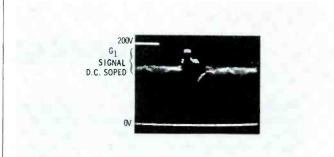
Fig. 12. DC levels at AGC grid.
