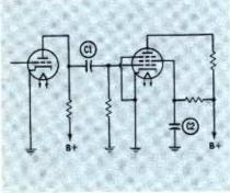
Fig. 1. Small-value coupling and bypass capacitors in a typical R-C amplifier.
