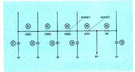
Fig. 2. Ohmmeter tests in this B+ feeder string quickly pinpoint exact fault.
