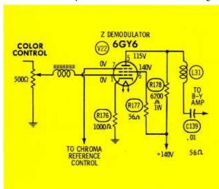
Fig. 2. Admiral 24E2 Z demodulator circuit.
