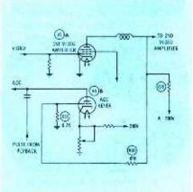
Fig. 4. Source of cathode voltage.
