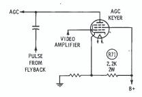
Fig. 10. Source of screen voltage.
