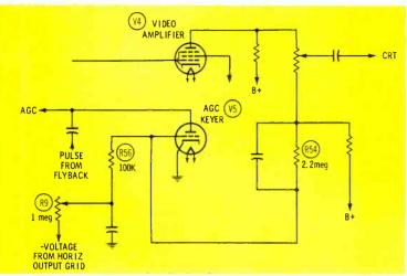
(V7) VIDEO VIDEO DETECTOR AGC (V8 V6 B SYNC SEPARATOR AMPLIFIER
