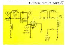
Fig. 9. Bad V6 produced odd symptom
