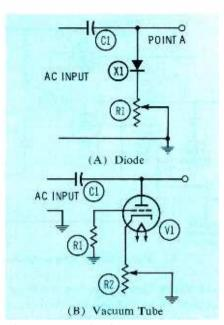
Fig. 2. Control of rectified voltage.
