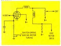
Fig. 8. Cathode lead opened during automatic tuning.
