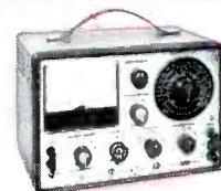
New Model 965 FaradOhm Bridge/Analyzer. "Unusually versatile" — Electronics World. 9-range, low-voltage capacitance-resistance bridge safely measures even 1-volt electrolytics. Metered bridge balance, leakage test voltage (6 DC VTVM ranges 1.5-500V), leakage current (11 DC VTAM ranges 0.15ua-15ma). DC VTVM & VTAM externally usable. $129.95 wired.
