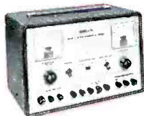
New Model 1030 Regulated Power Supply. Speeds troubleshooting, design work, production line testing, electronics teaching. Variable bias and plate sources regulated to 1/3 of 1%: 0-150V @ 2ma; 0-400V @ up to 150ma. Ripple less than 3mv rms. Unregulated fil. volts of 6.3V & 12.6V, @3A. Switchable, monitoring milliammeter and voltmeter. $59.95 kit, $99.95 wired.
