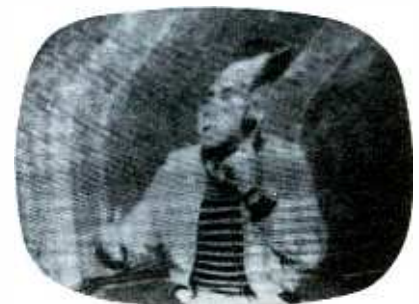
Fig. 5. Twist caused by distorted sync.
