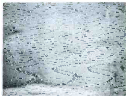
Fig. 15. Random noise due to arc inside 6BK4 plate cap.
