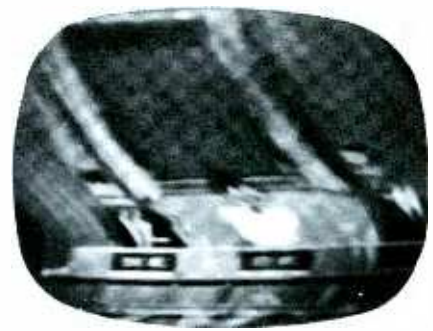
Fig. 8. AFC trouble causing twist.
