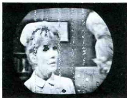
Fig. 14. Noise due to arc inside 3A3 plate cap.
