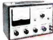
New Model 378 Audio Generator. Near-distortionless sine wave generator (<0.1% 20-20,000c) providing fast, convenient switch-selection of frequencies from 1c to 110kc (1c steps 1c-100c, 10c steps 100c-1kc, 100c steps 1kc-10kc, 1kc steps 10kc-110kc). 8-pos. 10db/step output attenuator & fine attenuator. Output meter (4 1/2" 200ua) with 8 voltage ranges & db scale. $49.95 kit, $69.95 wired.
