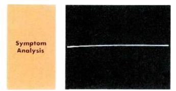
Narrow horizontal line through center of screen indicates absence of vertical sweep. Vertical linearity or size controls have no affect on bright horizontal line. Turning vertical hold produces no change. Rotation of controls renders no helpful hints.
