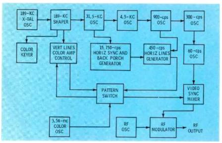
Fig. 2. Block diagram reveals signal paths of complete solid-state color generator.
