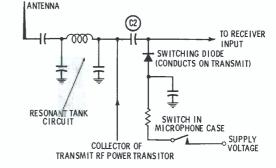
Fig. 10. Electronic antenna switching using a diode.
