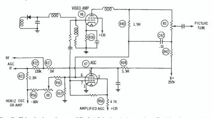
Fig. 7. This single tube amplified AGC circuit is used in Zenith Chassis 17Z30.
