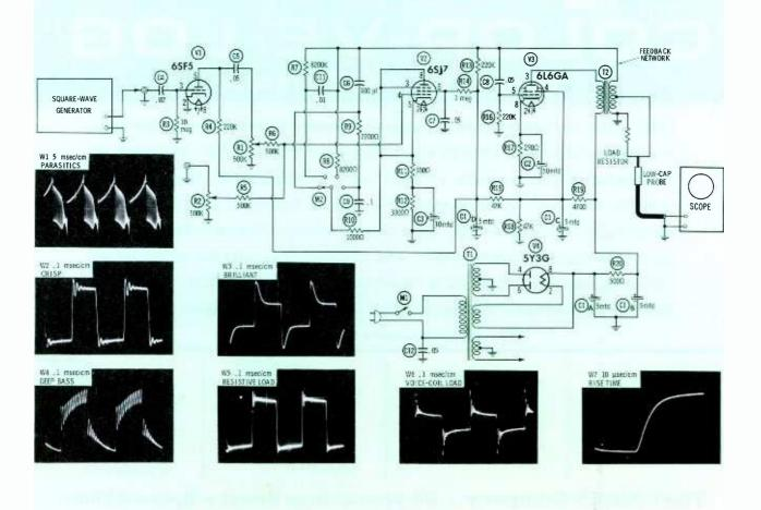
Fig. 2. Utility amplifier commonly used for public-address systems provides better reproduction than the two-tube type. 32 PF REPORTER/February, 1966
