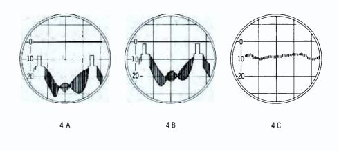
Fig. 4. Waveform as it appears at grid and cathode of AGC amplifier V15A.
