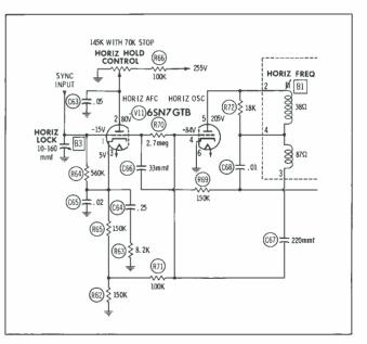
It sounds as though a component, probably a capacitor, is breaking down due to heat. This occurs only when the chassis is in the cabinet because the components are exposed to a lower temperature if the set is operating on the service bench. With the set on the bench, you can use a heat lamp, directed toward the chassis, to simulate the heat conditions that exist within the cabinet.
