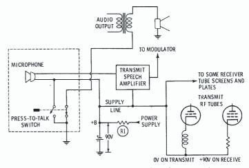
Fig. 4. Alternate direct switching method for transceivers.
