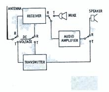
Fig. 2. Transceiver switching operation.
