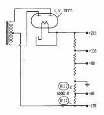
Fig. 6. Observe power-supply voltages.
