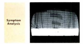
Picture up one-third from bottom and appears to have foldover and multiple images. Vertical scanning uneven with top half of screen extremely stretched. Vertical hold will sync picture; however, vertical height and size controls have no effect on raster.
