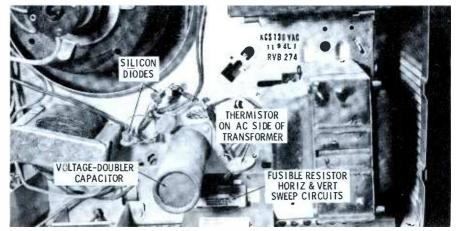
Fig. 3. Location of low-voltage power supply components used in an RCA portable.
