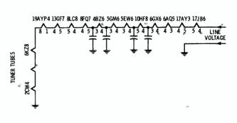
Fig. 2. Series filament circuit in modern-day receivers.
