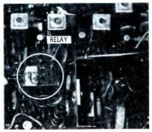
Fig. 7 Note relay on printed board.
