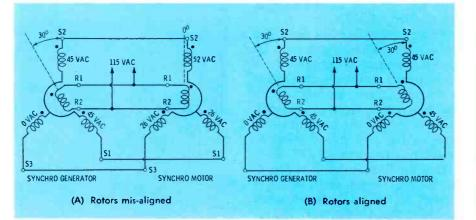
Fig. 5. High current flows until both rotors are aligned-residual current remains.
