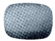
Fig. 9A. No picture—lines in raster.
