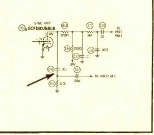
Mfr: Motorola Chassis No. QTS-576Y TO AGC -FROM H.O.T. AGC KEYING SYNC SEP NOISE LIMITER FROM VIDEO FROM Card No: MO QTS576-2 OUT DFT (V5) 3BU8 -1.5V TO SYNC AMP Section Affected: Picture and sync. 8 230V 135 140V FROM VIDEO OUT Symptoms: Video overload; erratic horizontal 180V FROM and vertical hold. H.O.T. Cause: Noise-Gate control defective. (R31) \$ 220K What To Do: Replace Sync-Stabilizer (Noise-(R8) NOISE GATE Gate) control R8 (4 meg). 245V (SYNC STABILIZER)
