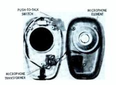
in both transmit and receive modes. This necessitates audio amplifier input-output and microphone-loudspeaker switching operations. Secondary switching operations may involve circuits such as squelch, tone control, speech amplifier, etc.
