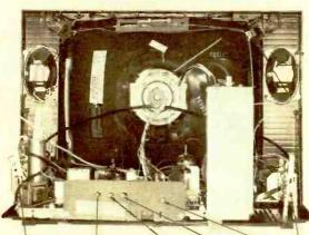
VHE TUNER VERTICAL LINEARITY HEIGHT HORIZ HOLD WIDTH UHE TUNER
