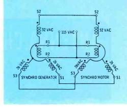
Fig. 4. Diagram shows connections. that the rotor can align itself  $180^{\circ}$  out of position.
