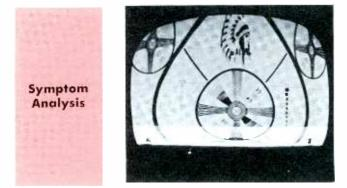
Vertical hold will sync picture but does so near one end of its rotation. Attempt to adjust height and linearity controls prove fruitless and produces uncontrollable loss of vertical sync. Very pronounced foldover present at bottom of picture.
