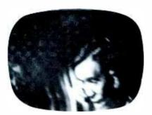
Fig. 1B. Overloaded picture from AGC
