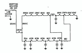
Fig. 1. Early model TV's used a series-parallel circuit.
