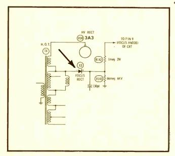
Mfr: G. E. Chassis No. CY (Color) Card No: GE CY-6 Section Affected: Raster. Symptoms: Proper focus cannot be obtained. Cause: Focus rectifier shorted. What To Do: Replace focus rectifier X3.
