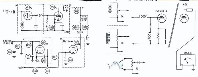
Fig. 2. Amplified-AGC circuit used in early model RCA's. Fig. 3. How AC and DC potentials affect video amplifier.
