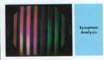
Monochrome picture is deep green or chartreuse. Tint and color controls do change intensity and position of color bars from generator; but blue bars are missing — only green and red visible. Chroma-output or CRT trouble is most likely.
