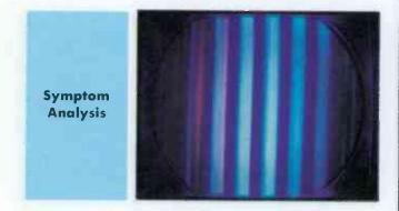
Green content of flesh tones is visible only with tint control fully clockwise; normal setting makes flesh magenta. Monochrome picture turns magenta at low brightness setting. Symptom indicates gray-scale misalignment or chroma-output circuit trouble.
