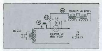
Fig. 6. Bad thermistor causes too much current in coils.
