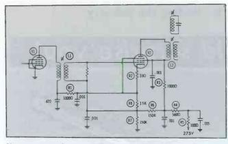
Fig. 2. First video-IF receives B+ from cathode of second.
