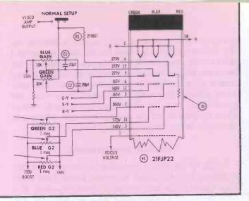
Fig. 2. Interelectrode leakage affects gray-scale adjustment.
