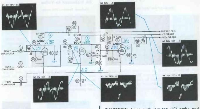
DC VOLTAGES taken with VTVM, on inactive channel; antenna terminals shorted. \*Indicates voltages with signal present — see "Operating Variations." WAVEFORMS taken with low-cap (LC) probe and wideband scope synced from blanking-amp cathode. All TV controls are set for normal color-bar pattern.
