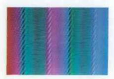
Fig. 10. Trap causes ringing in video, creates changes in chroma channel.
