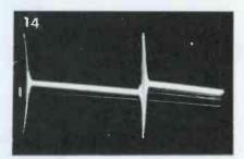
detectors. A burst-amplifier transformer with center tap develops the two opposite phases of 90-volt burst in photos 13 and 14, which are shown as they are applied (through 330-pf capacitors) to the chroma-sync phase detector. The same signals are applied to the killer phase detector, also through 330-pf capacitors.
