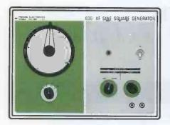
MODEL 636 AF SINE SQUARE GENERATOR – 20 cps to 200 kc in four ranges. Less than 0.25% sine wave distortion at 10 vrms into 600 ohms load.
