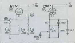
Fig. 10. Changing bias-operated contrast circuit to a variable-degeneration.
