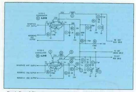
Fig. 4. Shorted C5 removes screen-grid voltage, tube and conduction ceases.
