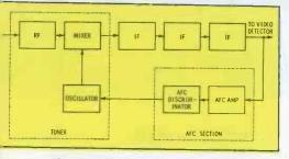
Fig. 1. AFC system is merely feedback loop for correcting oscillator drift. discriminator, receiving this higher IF carrier, would develop a positive correction voltage. If the oscillator drifted downward in frequency, or if the fine tuning were incorrectly set to a frequency slightly lower than normal, a lower video IF carrier would be generated, and the AFC discriminator would produce a negative correction voltage.
