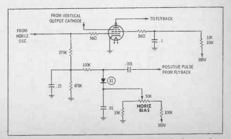
Fig. 14. Motorola TS914 uses sweep regulation instead of high-voltage regulator.
