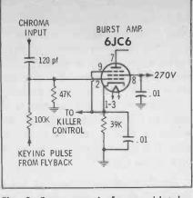
Fig. 8. Burst amp is frame-grid tube.
