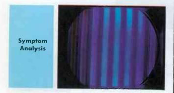
With brightness control at maximum setting, screen still is dim for both color and black-and-white pictures. Bar at far right should be green; instead, is dark blue and barely visible. Absence of a color indicates trouble in chroma, not luminance, circuits.
