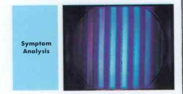
Black-and-white picture is tinted blue. At normal position of tint control, flesh tones are green; with control fully counterclockwise, they are weak magenta. Color-bar pattern proves red output is weak indicating gray-scale misalignment or chroma-output trouble.
