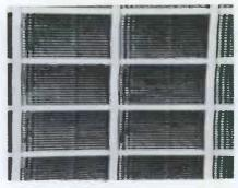
Fig. 6. Ringing in certain b-w sets with high-level video pot. Tuning is no help.
