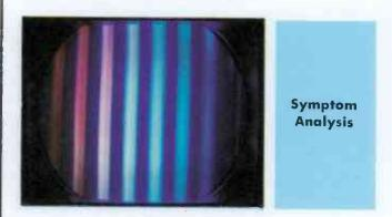
Red content of color picture is smeared and faded; fine-tuning control won't correct trouble. Black-andwhite picture shows no evidence of smear or ringing. Color-bar pattern also shows red smear. Other colors are okay, clearing video-IF, chroma-bandpass circuits.
