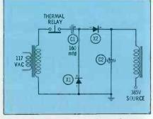
Fig. 1. Doubler circuit, thermal cutout.
