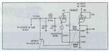
Fig. 7. Vacuum-tube-voltmeter reading will not exceed full scale.
