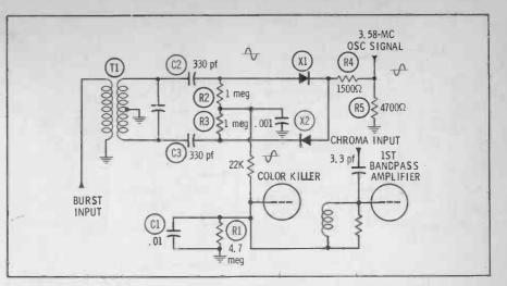
Fig. 4. ACC voltage governs gain of bandpass amplifier in this Philco design.
