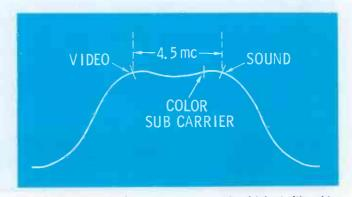
Fig. 1. The VHF-tuner response curve should look like this.
