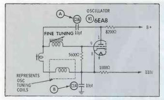
Fig. 7. Defective C16 changes VHF oscillator frequency.
