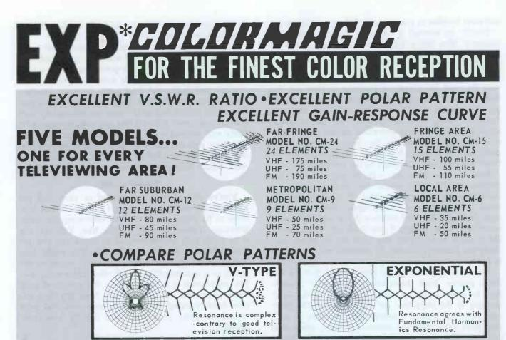
**V-TYPE:** Antennas have polar patterns similar to that shown above. Notice the large side lobes on the polar graph. These lobes indicate distorted reception-the cause of impure color and ghosting.
