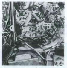
Loose connection on burst transformer.
