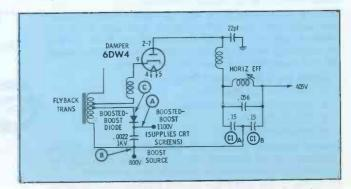
Fig. 1. Rectified positive flyback pulse is added to boost.
