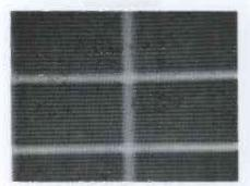
Fig. 4. Dullness in this pattern results from misadjustment of fine-tuning.
