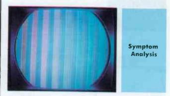
Picture blooms, retrace lines are visible, and brightness is excessive at normal control settings for both black-and-white and color reception. Color is weak, even with color control set for maximum. Washed-out color points to chroma-circuit defect.
