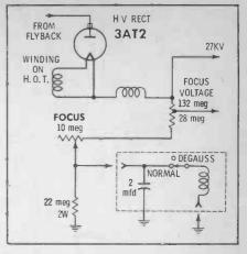
Fig. 13. Degaussing is in HV circuit.
