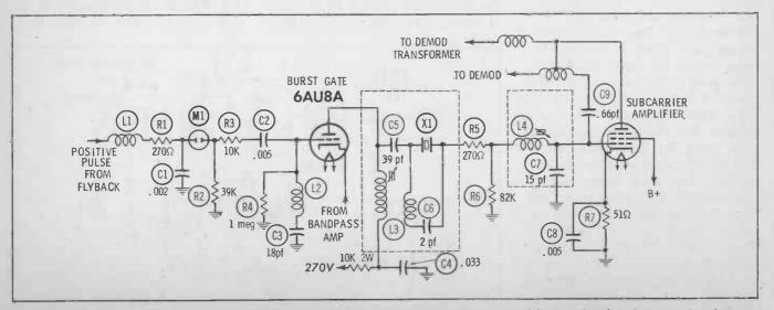
Fig. 7. General Electric's CB chassis uses ringing circuit and a subcarrier amplifier to develop 3.58-mc signal.
