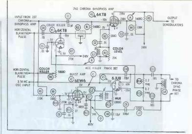
Fig. 8. Missing burst pulse caused killer to cut off bandpass.
