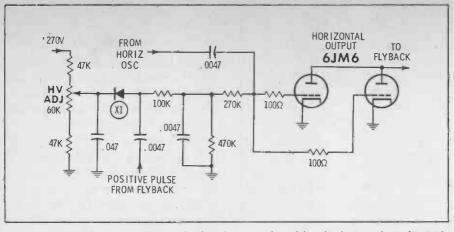
Fig. 12. High-voltage regulator tube has been replaced by diode in Admiral's G11.
