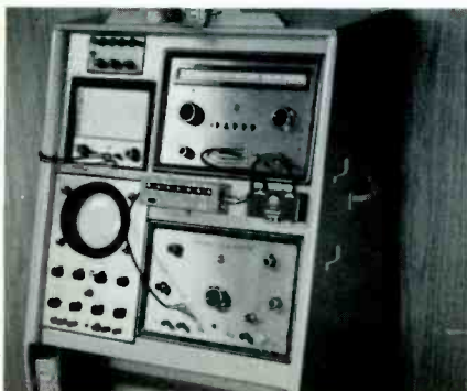
Fig. 1. Alignment equipment rack simplifies connections, and saves time.
