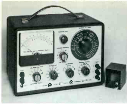
Fig. 3. This unit has a low range of .15 ua when in the DC VTAM Position.
