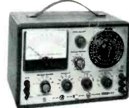
New Model 965 — FaradOhm Bridge/Analyzer. 9-range, low-voltage capacitance-resistance bridge safely measures even 1-volt electrolytics. Metered bridge balance, leakage test voltage (6 DC VTVM ranges 1.5-500V), leakage current (11 DC VTVM ranges 0.15ua-15ma). DC VTVM & VTAM externally usable. $129.95 wired.
