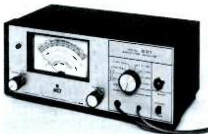
Fig. 1. Bridge-type analyst reads effective capacitance for electrolytics.
