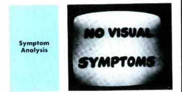
Normal volume is developed, but with volume control near maximum. High-frequency audio is slightly reduced. Symptom might suggest audio-circuit trouble, but any trouble there would generally cause more pronounced change.
