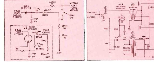
Fig. 5. Focus circuit for the 21" and 25" color receivers.
