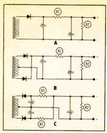
Fig. 3. Simple B- supply arrangement.
