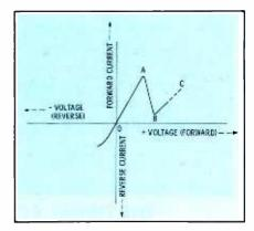
Fig. 3. Characteristic of tunnel diode.
