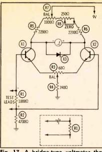
Fig. 17. A bridge-type voltmeter that uses differential-amplifier principles.
