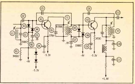
Fig. 13. These IF stages operate much the same as any solid-state RF amp.
