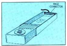
Fig. 8. Don't insert radio upside down.
