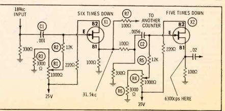
Fig. 28. Latest development for counting circuits is the unijunction transistor.
