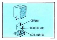
Fig. 5. Loose collar shifts frequency.
