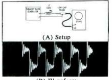
(B) Waveform Fig. 1. Ringing test for air-core coil.
