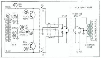
Fig. 3. Transistorized circuit replaces conventional vibrator.
