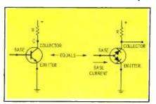
Fig. 1. Switch equivalent of transistor.
