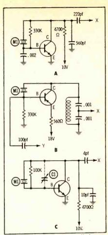
Fig. 22. Three crystal-controlled transistor oscillators of the Pierce variety.
