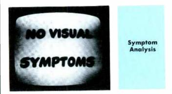
Normal volume can only be obtained by setting volume control almost to maximum. Since audio is so low at normal setting, noise and vertical buzz are heard with higher setting. Such noise is most likely to be picked up in stages where audio is weak.
