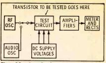
Fig. 19. Standard transistor circuits can be used to test other transistors.
