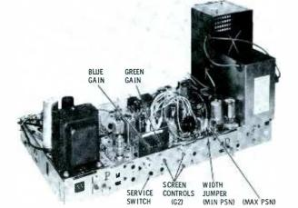
Fig. 1. Zenith's 25" color chassis contains a width jumper.
