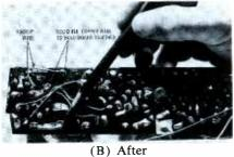
Fig. 6. Repair of broken PC board.
