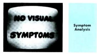
With volume control at maximum, slight buzz and background noise are heard; no audio signal is present. Since noise and buzz are heard from speaker, audio stages must be good. Noise is low in volume, so suspected stage is near end rather than near beginning of sound IF strip.
