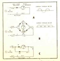
Fig. 1. Most common rectifier circuits.
