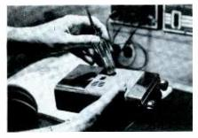
Fig. 6. Tapping case aggravates fault. Third IF Coil
