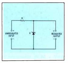
Fig. 2. Zener diode used as regulator.
