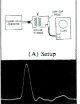
(B) Waveform Fig. 6. HF-inductor test.
