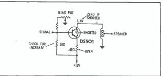
Fig. 13. Watch for these possible faults in power stage. 0 and 70 ohms when the leads are flexed.
