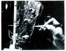
Fig. 5. Notice loose grounding eyelet.
