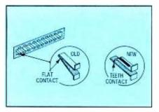
Fig. 2. New contact type solves fault. 42 PF REPORTER/June, 1965
