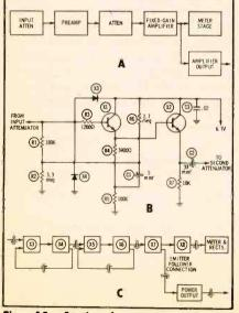
Fig. 18. Sectional arrangement and preamp schematic of audio voltmeter.
