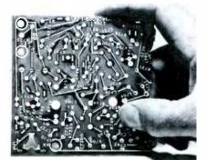
Fig. 1. Backlighting reveals wiring.
