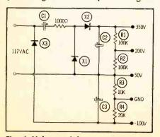
Fig. 4. Voltage tripler; note GND point.
