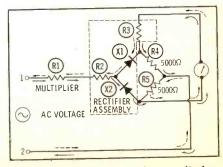
Fig. 2. Full-wave with only two diodes.
