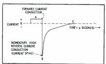
Fig. 8. PIN-diode characteristic curve.
