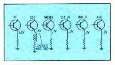
Fig. 7. Emitter test for open transistor.
