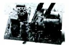
Fig. 3. "Looping" new part to board.
