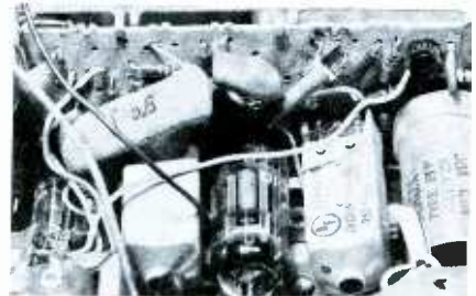
Fig. 2. Lift one end of the base resistor (this is 5.6 ohms) for test.
