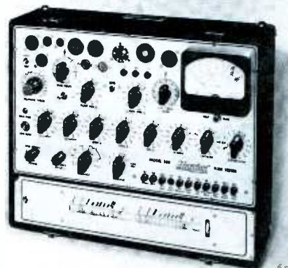
Fig. 5. This tester checks tubes using roll-chart or tube-handbook data.
