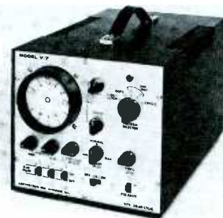
Fig. 9. Simple scope provides a way to view the vector relationships.
