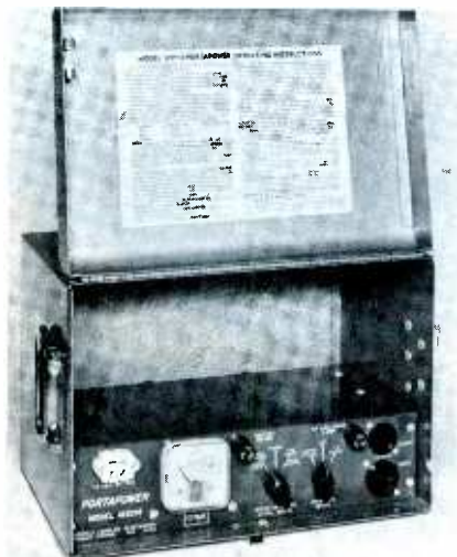
Fig. 1. This DC-to-AC converter also has provisions for recharging its battery from AC.
