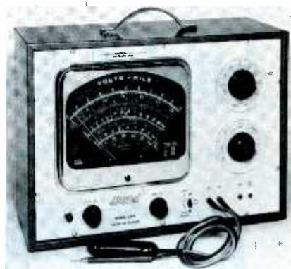
Fig. 3. VTVM features measurement ranges for current, voltage, resistance, capacitance.
