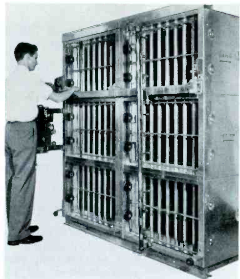
Fig. 4. Large units are installed in the air-circulating systems of commercial buildings.
