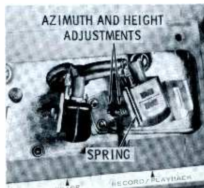
Fig. 5. A typical side-mounted head assembly.
