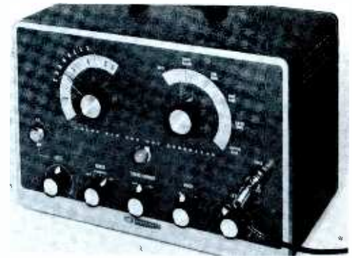
Fig. 2. This color generator produces dots, crosshatch, and vertical and horizontal bars.
