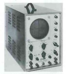
Fig. 1. Wideband scope includes frequency compensated vertical amplifier.
