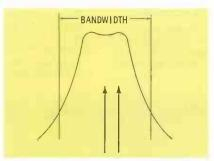
Fig. 2. Misalignment will widen bandwidth and ruin receiver selectivity.
