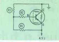
Fig. 2. Since a transistor is solid-state, it has resistance between electrodes.
