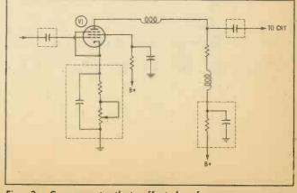
Fig. 3. Components that affect low-frequency response.
