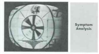
Visual indications are approximately same as in Symptom 2—picture pulls away from right edge of screen and may show phasing ghost at left. Attempt at correction makes sync less stable. Horizontal bending of picture varies with program material.
