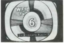
(A) Video 50V p-p (B) Video 75V p-p (C) Video 100V p-p Fig. 3. Visual effect on picture contrast as video signal amplitude varies.
