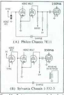
Fig. 12. Twist was caused by bad 25DN6 in circuit A, but not in circuit B.
