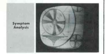
Picture remains fairly steady (though jittery) with horizontal blanking bar visible near either left or right side of screen. Bar can be "flipped" to one side or the other with L1, but attempt to adjust for normal phasing always causes complete loss of sync.
