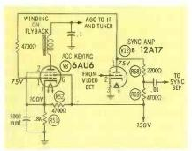
Fig. 1. Input to AGC tube in Westinghouse V-2313 is from a sync amplifier.
