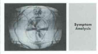
On local channels, keyed AGC cuts in and out of operation when L1 is adjusted, causing violent shaking of picture. Weak signal gives steadier picture, but is still troubled by intermittent horizontal bending and loss of sync on signal interruptions.
