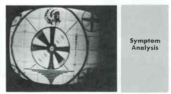
Picture locks in solidly, but L1 needs readjusting when set is turned on, and again after thorough warmup. Tipoff to phasing fault is visible black border at right of screen, and milky phasing ghost at left. Attempt to correct it throws picture out of sync.
