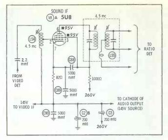
coupled into the sound circuits through faulty lead dress, or by leakage in the socket of V8 from the triode section (sync phase inverter) to the pentode section (sound IF).
