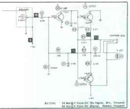
Fig. 4. Common-collector outputs use this hookup to obtain operating bias. ances extending from the 9-volt source to ground (X4 collector). Likewise, X4 and X5 base voltages are the result of divider action. (Notice that the collector of X3 and the base of X4 are DC coupled. This is possible because X3 is a PNP and X4 is an NPN.)
