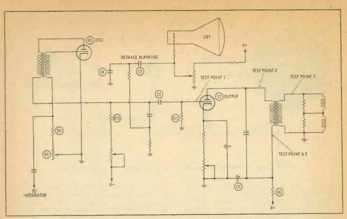
Fig. 1. Common blocking oscillator circuit used in a number of older receivers.
