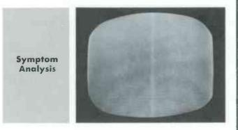
Trouble looks like blocked IF due to loss of AGC. Disconnecting antenna or switching to weak station brings in picture, but horizontal sync is very unstable. Grounding grid of V2 restores normal sweep and lets keyed AGC circuit operate properly, restoring video.
