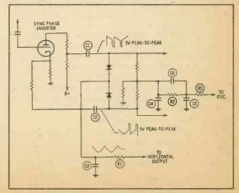
Fig. 5. An example of a dual-diode horizontal AFC circuit.
