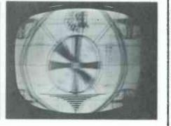
Multivibrator reacts normally to grid-grounding test. When ground lead is removed, AFC throws multivibrator off frequency. Sync can be restored by backing out L1 slug, but is extremely critical—picture soon begins to jitter, and falls out of sync.
