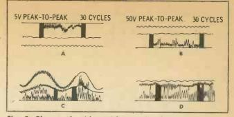
Fig. 2. Plate and grid waveforms of video output stages.
