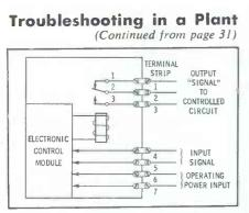
Fig. 8. Terminal strip simplifies the troubleshooting of this control device.
