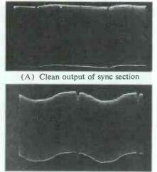
(B) Hum in AFC sample signal Fig. 11. Sync waveforms in Philco 7E11 when faulty 25DN6 was installed. the horizontal twist was a thing of
