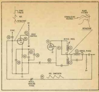
Fig. 4. Waveforms and controls in Synchroguide stage.
