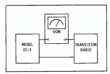
Fig. 4. Test setup for checking meter.
