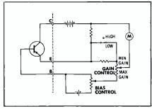
Fig. 7. Simplified diagram of gain test.
