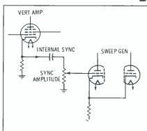
Fig. 7. Sync signal is coupled from vertical amplifier to sweep generator.
