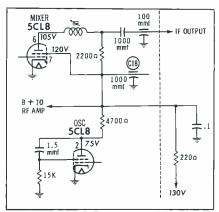
Fig. 5. Too-low value of C18 and other bypass capacitors can cause troubles.
