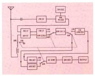
Fig. 3. FM section of Bendix includes limiter stage.
