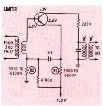
Fig. 4. Values of R1 and R2 are chosen to provide effective limiting action.
