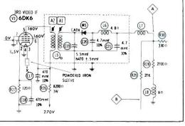
Fig. 6. Video detector circuits are usually shielded to prevent radiation.
