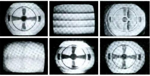
Fig. 1. These six symptoms are only a sample of IF-regeneration troubles.
