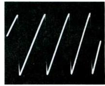
Fig. 2. Virtually pure sawtooth shape characterizes sweep-generator output.
