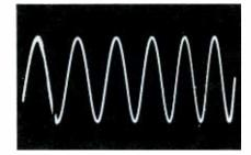
Fig. 5. Nonlinear horizontal sweep is demonstrated by uneven waveform. injection signal is needed to give the most readily understandable results. To evaluate the output, simply display a single cycle of a sine-wave audio signal on the screen and carefully compare the width of the two half-cycles as shown in Fig. 6. Distortion of the sawtooth waveform causes unequal distances between
