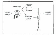
Fig. 4. Wide-band scopes use peaking coils to broaden the vertical response. so normal overloading won't be introduced.) When the waveshape on the screen becomes distorted, you've found the distortion-producing stage.
