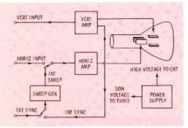
Fig. 1. Scope circuitry can be divided into four major sections for analysis.
