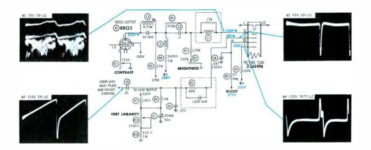
DC VOLTAGES taken with VTVM, on inactive channel; antenna disconnected from set. \*Means voltage varies with conditions—see "Variations."
