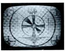
Brightness control must be advanced nearly to full clockwise setting for normal brilliance. White retrace lines may be present in all parts of picture, or only in small area near top; in any case, they are almost sure sign of trouble in CRT grid circuit.
