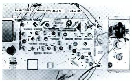
Fig. 4. Certain major components are located on top of chassis.
