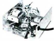
Fig. 3. Screwdriver control sets meter.
