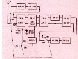
Fig. 5. Delco AM-FM circuit incorporates separate oscillator for AM only.
