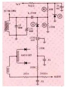
Fig. 2. Variable-capacitance diode X1 is key component in FM AFC circuit.
