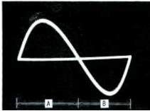
6. Distortion of sawtooth sweep will produce unsymmetrical sine wave.
