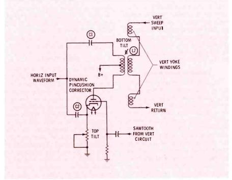
Fig. 3. Special circuit is used to offset pincushioning in 92° pic tube.
