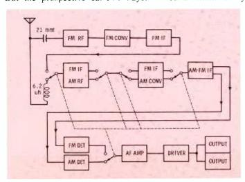
Fig. 1. Automatic's AM-FM radio has four FM IF's.
