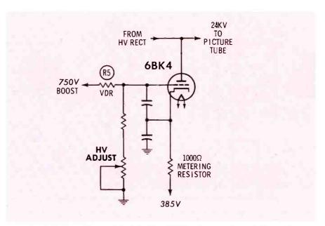
Fig. 2. Grid of HV regulator tube has VDR for improved regulating action.
