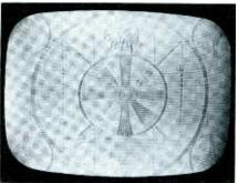
Since contrast and brightness controls operate properly, and picture detail is sharp, CRT is probably okay. Picture contains no snow, so low gain in video output stage is most likely fault—although possibility of weak IF or too much AGC shouldn't be dismissed.
