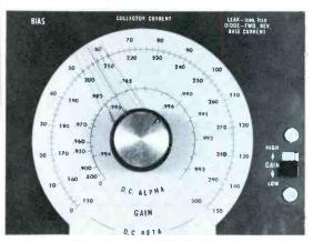
Fig. 8. Gain dial includes two scales.
