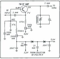
Fig. 6. Delco's AGC circuit uses two diodes operating as voltage doubler.
