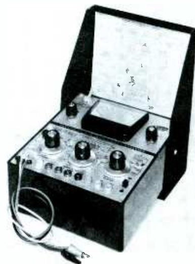
Fig. 4. Unit can test many different kinds and types of semiconductor units.
