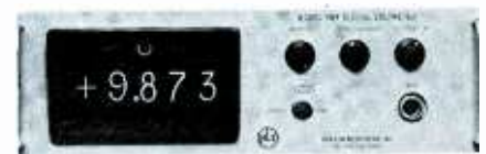
Fig. 3. Digital voltmeter generates voltage to compare with unknown.
