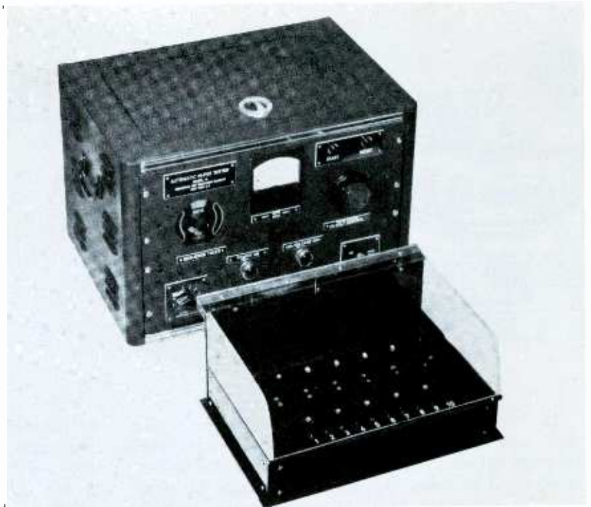
Fig. 2. Hi-Pot tester locates breakdowns in insulation between conductors.
