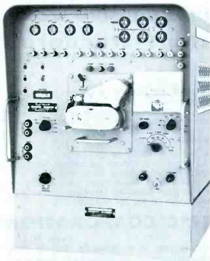
Fig. 7. Robotester automatically performs tests programmed on a tape.
