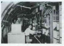
Inside of flying TV station, with engineer operating two-channel console.
