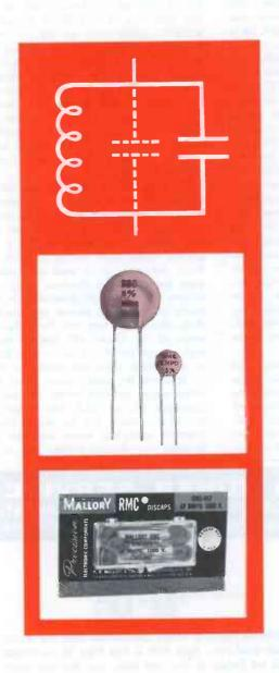
While an oscillating circuit is warming up, its frequency changes. Distributed capacitance in tubes and coil will drift in the "positive" direction—tending to decrease the resonant frequency. Unhappily, the tuning capacitor, if it is a conventional mica or paper unit, also drifts in this same direction . . . thereby adding to the downward frequency shift.
