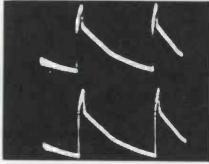
(A) Sawtooth modulating voltage.
