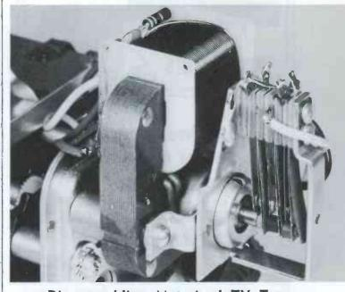
Dissassembling Motorized TV Tuners When you remove the motor, gears, and switches to make way for tuner repairs, you'd better note how they fit together.
