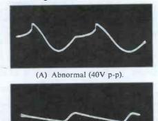
(B) Normal (15V p-p).Fig. 4. Ripple at point M.
