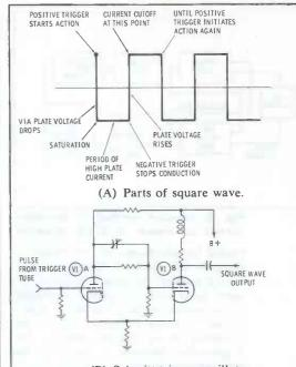
(B) Schmitt-trigger oscillator.
