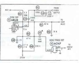
only waveform trouble is at the screen of the 6BU8; the scope trace looks fuzzy instead of having the shape shown on PHOTOFACT. Both horizontal and vertical hold are critical. Can you help?
