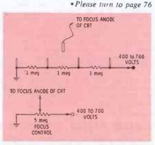
Fig. 3. Most modern receivers use one of these circuits for focusing the CRT.
