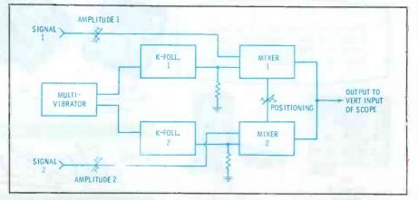
Fig. 2. Block diagram shows circuits that combine signals and switching.
