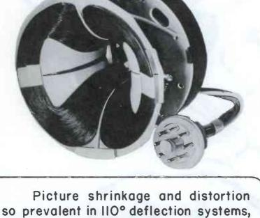
so prevalent in IIO° deflection systems, is generally caused by excessive heat, which expands and contracts the windings of a deflection yoke......MERIT solved this problem "once and for all."
