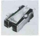
A series of ceramic replacement stereo cartridges, having a dual stylus for playing either stereo or monaural records, is now available. Made by Euphonics, the U-8 and U-9 feature a tracking force of 2 grams and high compliance. The U-8, with the sapphire dual stylus, carries a list price of \$9.95. The U-9, with a .0007" diamond and .003" sapphire stylus, lists for \$14.95.
