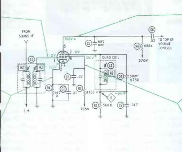
DC VOLTAGES taken with VTVM, on inactive channel, with antenna terminals shorted. means voltage will vary when signal is applied or control is adjusted. See "Variations."
