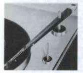
The Model M222 tone arm, which uses an N22D tubular stylus with a .0005" diamond point, is new from Shure. It has a tracking pressure of less than  $1\frac{1}{2}$  grams, frequency response from 20 cps to  $20 \cdot \text{kc}$ , channel separation of more than 22.5 db at 1000 cps, and output voltage of 4.5 mv. Audiophile net price of the M222, including the N22D stylus, is
