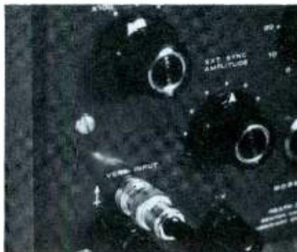
Fig. 5. Coaxial connectors installed in place of the binding posts on scopes.
