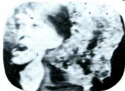
Fig. 12. Hum was mistakenly assumed to be the cause of this twisted picture.
