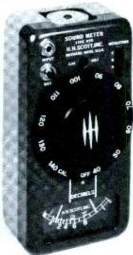
Fig. 4. Small-sized sound meter is useful for a large number of jobs.
