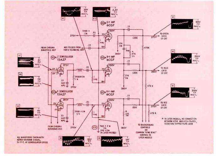
Fig. 1. Chroma demodulators and color-difference amplifiers of typical color TV (RCA Chassis CTC9).
