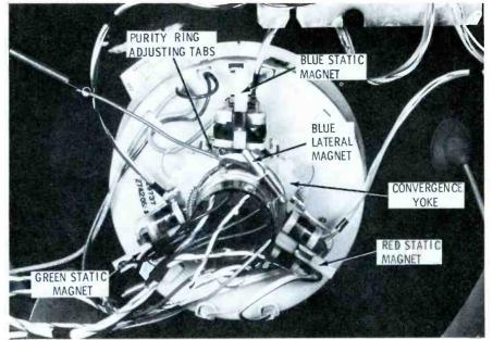
Fig. 1. Purity adjustments and convergence yoke are located on CRT neck.
