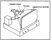
Fig. 3. Tin foil "patch" makes substitute for missing aquadag CRT coating.
