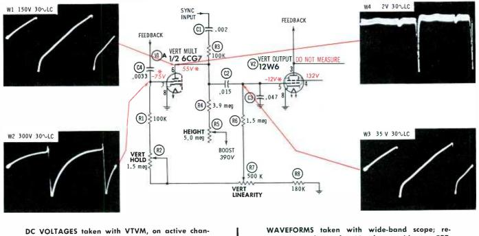
DC VOLTAGES taken with VTVM, on active channel. \* means voltage will vary when signal is applied or control is adjusted. See "Variations."
