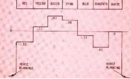
Fig. 2. Actual and theoretical G-Y waveforms of NTSC color-bar pattern.
