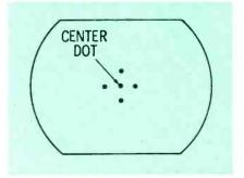
Fig. 2. Observe center dot while performing static convergence of beams.
