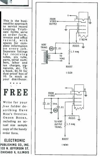
tion to this grid should be broken, and a 39K resistor in parallel with .01-mfd capacitor inserted between pin 2 and ground.
