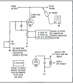
Fig. 2. Meters show the color-TV technician what's going on in HV circuits.
