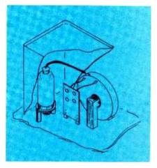
Fig. 1. Most common mounting for high-voltage sockets in older TV receivers.
