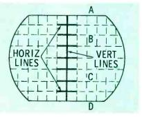
Fig. 3. Check for vertical dynamic convergence in this area of crosshatch.
