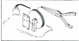
Fig. 2. Secondary winding of flyback transformer can sometimes be repaired.
