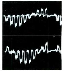
Fig. 4. Waveforms W4 and W5 applied to grids of R-Y and B-Y amplifiers. equally in the same direction; if they are, they can usually be brought back to normal by readjusting the hue control or the burstphase transformer. When only one or two nulls are out of place, the fault ordinarily lies in the demodulator-phasing adjustment or in one of the demodulator circuits.
