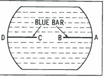
Fig. 4. Straightening the blue bar is first step of horizontal convergence.
