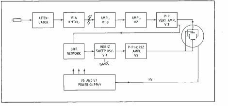
Fig. 4. Block diagram of PS120 scope.
