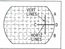
Fig. 5. Check convergence of both vertical and horizontal bars at right side.
