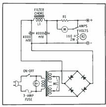
Fig. 8. Schematic showing straightforward circuit, special two-way meter.
