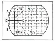
Fig. 6. Follow this pattern to adjust horizontal convergence at left side.
