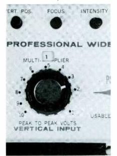
Fig. 2. Closeup of vertical attenuator showing multiplier reading in window.
