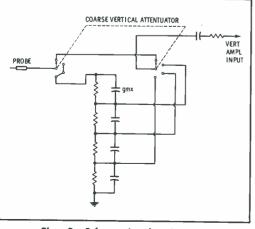
Fig. 3. Schematic showing compensation networks of vertical attenuator.
