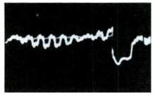
Fig. 5. W6 is developed across cathode resistor R178 in circuit of Fig. 1.
