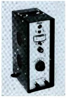
Fig. 6. Low-ripple DC supply can also be used for powering transistor radios.
