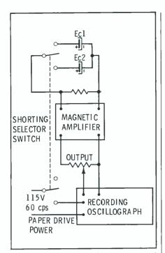
Fig. 4. A recording oscillograph is used to obtain an accurate measurement. time-response values which are in the order of several cycles at the supply frequency.
