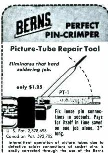
Intermittent operation of picture tubes due to defective solder connections at socket pins is easily corrected through the use of the Berns Perfect Pin Crimper. Actually a 3-in-1 tool that can also be used as a channel-selector wrench and screwdriver, it serves to notch pins and element leads to provide solid electrical connections. Pin keeps its original form.
