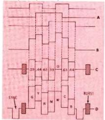
Fig. 2. Composite color signal consists of several components, pictured here.
