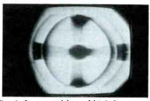
Fig. 6. Smear and loss of high frequencies, due to a defective peaking coil.
