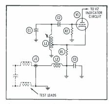
Fig. 7. An open circuit across the test leads causes V1 to stop oscillating.
