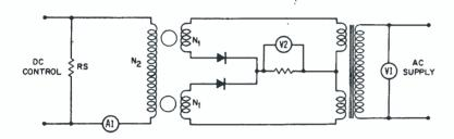
Fig. 1. Test arrangement for obtaining amplifier control characteristics.
