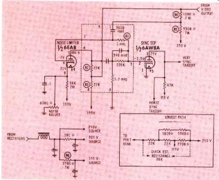
Fig. 1. Open path between the grid and ground caused pulling and poor sync.
