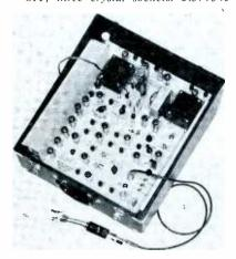
Fig. 1. Portable color generator is complex, with many tubes and adjustments.
