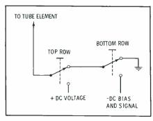
Fig. 10. Unique push-button arrangement provides DC to tube elements.
