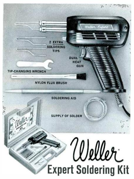
All your soldering needs in a break-proof plastic utility case. Gun features dual heat. 2 trigger positions permit instant switching to low 100-watt or high 140-watt heat. Low heat prevents damage to heat sensitive components. By using high heat only when necessary, you prolong tip life and save current.
