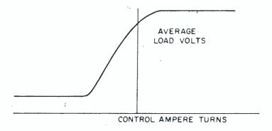
Fig. 2. Plotting load voltage vs control ampere-turns yields transfer curve.
