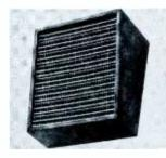
A new line of baffles and speaker - baffle combinations is announced by RMS Electronics. These wall-mount baffles are available with speakers (BS series) or without them (SB series), in sizes from 5" to 12". Cabinets are finished on four sides in mahogany, walnut or blonde. The decorator grille cloth is recessed ¼" from the front face of each baffle.
