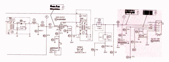
Fig. 2. Most TV receivers obtain adequate picture-signal gain from a one-stage video amplifier.
