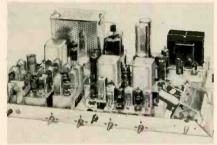
The latest revision of the deluxe unitized chassis carries the same number (X162) as last year's version. All circuits except the low-voltage power supply are mounted on six plug-in subchassis units.
