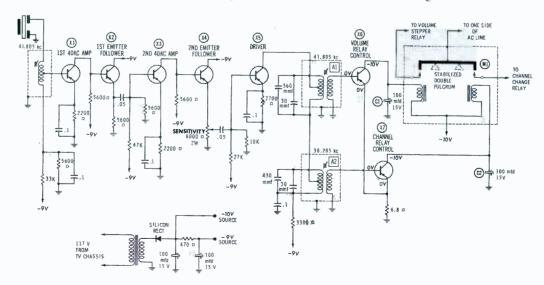
Fig. 2. Received signal is amplified to high enough level to drive relay-control transistors into conduction.
