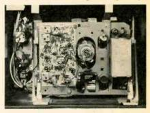
The chassis has one large printed board, marked with "road map" lines on the component side, and with See-Matic component symbols on the wiring side. In 19" models, the chassis can be pivoted back (after several screws are removed) and operated in a horizontal position.
