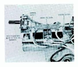
Fig. 3. Transistor collector current energizes one side of relay at a time.
