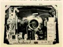
The deluxe "N" series continues to be used in high-end 23" models, retaining such features as a power transformer, 110° picture tube, keyed AGC, and 6DS4 nuvistor RF amplifier.
