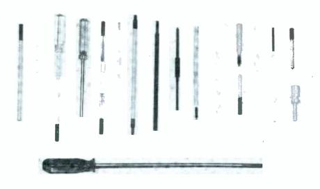
Fig. 2. Radio-TV service shops have uses for all these alignment tools.
