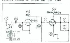
Fig. 5. Shorted capacitor across J1 removes cutoff voltage from grid of V1.
