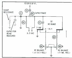
Fig. 8. When bridge circuit is balanced, capacitance is shown on the dial.
