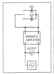
Fig. 3. Long time-constants are measured with a stop watch and indicator.
