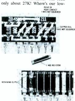
Fig. 2. Special printed component board used in noise-limiter and sync stage.
