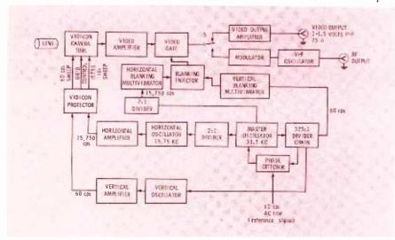
Fig. 2. Block diagram of camera using vidicon tube, showing circuit layout.
