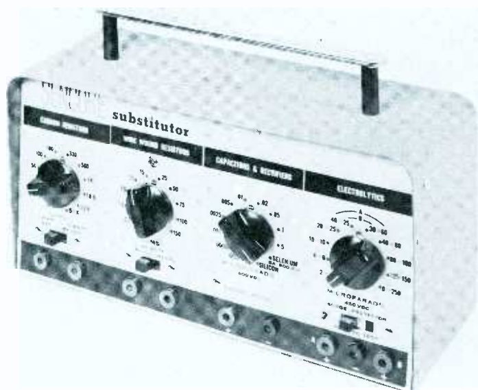
Fig. 1. New instrument substitutes components in many electronic circuits.
