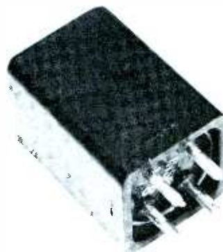
Fig. 7. Thermostatically - controlled ovens keep crystal temperatures even.
