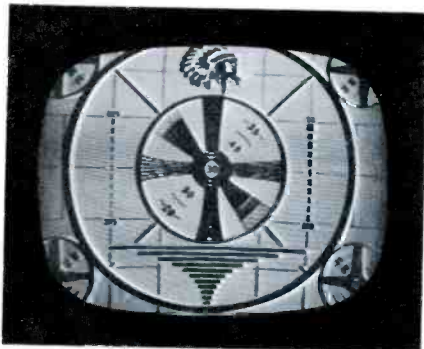
Fig. 2. "Trailing reversals" are due to phase distortion at low frequencies.
