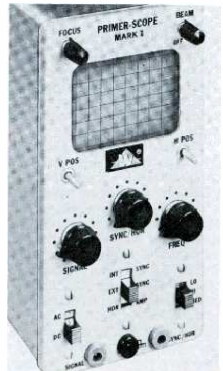
Fig. 3. Face of the Mark I has calibrated 3" screen and simplified controls.
