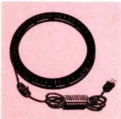
Fig. 1. Use of degaussing coil is first step in correcting poor color purity.
