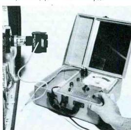
Fig. 3. Mercury's CRT tester restores emission and corrects other defects.
