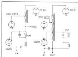
Fig. 5. Direct-drive and autotransformer flybacks have similar boost circuits.
