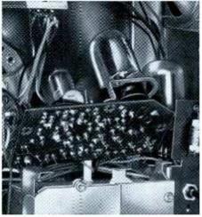
WP Sweep circuit board lifts up, to make component replacement fast and easy. Full fillet solder connections for sure contact.
