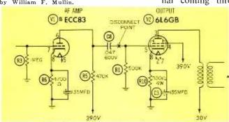
Fig. 1. Typical audio-amplifier circuit. grid-coupling capacitor
