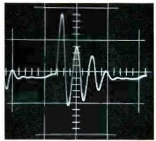
Fig. 4. Undamped oscillations at the damper are sure sign of boost trouble. and secondary of an isolated-secondary transformer.
