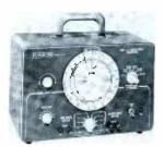
Paco Model generates both sinusoidal and square waves at any frequency between 6 cps and 750 kc. Maximum output obtained across a 600-ohm load is 10V rms for sine waves. or 18V p-p for square waves: amplitude is controlled by an attenuator switch and potentiometer. Rise time of square waves is less than .15 usec. Frequency accuracy is  $\pm 5\%$ .
