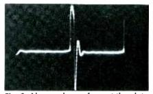
Fig. 8. Abnormal waveform at the plate (pin 5) of 6SN7GT in circuit of Fig. 7. hold adjustment was more critical
