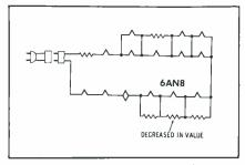
Fig. 4. Shunt resistor changed value, lowering filament voltage on one tube.
