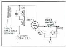
Fig. 2. Looking at only the boost circuit shows it to be a half-wave rectifier.
