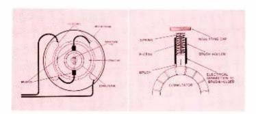
An appliance-motor commutator (arrow) should have a shiny ring all the way around. A rough, pitted surface usually indicates had brushes or an open armature coil. To clean and smooth a commutator, use very fine sandpaper (not emery cloth!) Brushes may groove the commutator; however, if its surface is smooth, spacers are intact, and brush springs have enough tension, the motor should still work properly.
