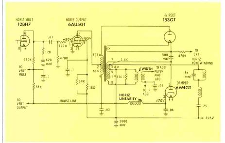
Fig. 1. Typical horizontal sweep section appears to be a complicated circuit.
