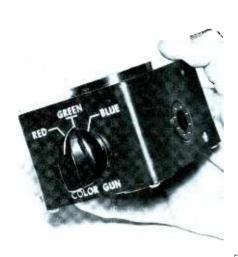
Fig. 4. Test head eliminates the need for additional test-socket adapters.
