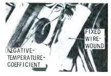
Fig. 1. Combination of two resistors protecting a series filament circuit.
