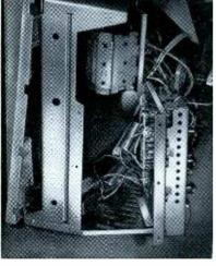
**OPEN** Precision-crafted IF circuit board swings open—components and connections are easy to get at.
