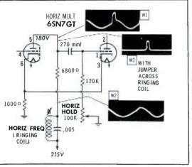
Fig. 7. Continuously-present fault in this stage behaved like warm-up problem.
