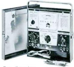
Tests all transistors in-circuit or out-of-circuit
