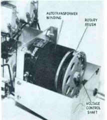
Fig. 2. Unusual transformer in the Model 1073 uses a rotary brush-type tap.
