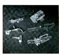
Irons, coffee makers, toasters, cookers, and other heatproducing appliances generally incorporate a small thermostat—a switch automatically activated by a heating element or by changes in ambient temperature. If you suspect thermostat trouble, inspect the switch contacts and look for corrosion or physical damage. Several adjustable types from electric irons are pictured here.
