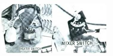
A faulty manual switch can cut off power to an appliance or cause intermittent operation. A continuity test with an ohmmeter will usually pinpoint this trouble. However, on heavy-duty switches, always check for high-resistance connections and signs of overheating.
