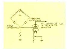
Fig. 4. Simplified bridge circuit employed to measure capacitance value.
