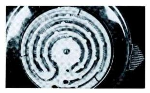
A heating element can carry enough current to produce usable heat energy without damage to the conductor. A continuity test or wattage measurement will quickly tell you its condition. Elements, if accessible, can be replaced by standard heating-element wire. Many appliances, however, employ a sealed unit. If open or shorted, this type must be replaced with an exact duplicate.
