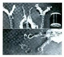
When replacing asbestos heavy-duty cord, remove about 3" of the outer coating, fold back the asbestos, strip the ends of the wire, and attach the connectors. Then, as a finishing touch, replace the asbestos and bind it with thread.
