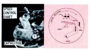
The speed of some motors is controlled by varying the applied voltage, while others use this centrifugal regulator. When the motor starts, the weighted arm moves away from the center axis; this, in turn, causes the motor-power contacts at A and B to break. The motor then slows down, but the spring soon pulls the arm in again and the contacts are closed. A capacitor (shown in photo) is usually placed across the contacts to reduce sparking.
