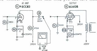
Fig. 2. Test procedure for leakage. Only ground return is through meter.
