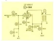
Fig. 3. Typical video-IF stage of a TV receiver. Note screen-bypass cap C4.
