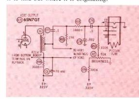
Fig. 2. Interfering signal can reach the CRT through retrace-blanking circuit.
