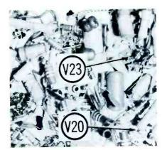
Fig. 2. Vertical position of chassis let melted wax run into tube sockets.
