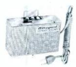
The amplifier circuit in the Winegard AT-6 "Booster-Pack" broadband TV-FM amplifier. using a low-noise MADT transistor, develops a gain of 16 db on the low VHF band and 14 db on the high band. A threeposition switch selects full gain. reduced gain, or amplification of signals picked up on the line cord in strong-signal areas. The unit obtains AC power through an isolation-transformer supply. List price is \$34.95.
