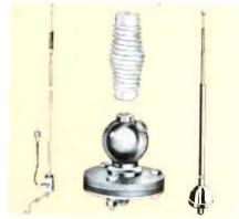
Mobile installations normally use quarterwave whip. For low-frequency operation, loading coil (in series with antenna or wound over it) extends electrical length. Swivel and spring mounts simplify attaching large antenna to vehicle.
