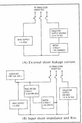
Fig. 6. Special in-circuit tests.
