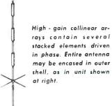
vertical collinear arrangement maintains a fully omnidirectional horizontal pattern, but further sharpens the vertical directivity pattern. The gain of the resultant antenna is a function of the number of collinear elements added. Practical gains as high as 10 db can be obtained in this type of system.
