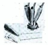
The tip of the Mueller "Micro-Gator" test clip has jaws 1/32" wide, with a 7/32" maximum spread. This clip, available in cadmium-plated steel or solid copper, can be soldered onto #20 or smaller wires and crimped in place with strain-relieving ears. Sold separately are skin-tight, flexible vinyl insulators, which cover the entire clip, but are split at the tip to allow the jaws to open.
