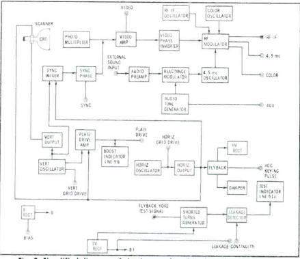
Fig. 3. Simplified diagram of circuitry employed in the Television Analyst.
