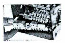
6. Tuner designed for quick, easy UHF conversion on the spot. You can convert tuner to take up to 4 UHF stations, switch strips without disassembling tuner or drum.
