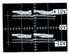
Fig. 6. Brightness control has this much effect on DC level of grid signal.
