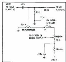
Fig. 4. Possible source of raster shading in the Philco Chassis 91 and J-1.
