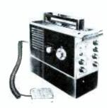
Transistorized except for two tubes in the transmitter section, the Vocaline "Commaire" Model PT-27 Citizens band transceiver operates from a rechargeable battery. The unit transmits on any four CB channels, while the receiver circuit includes a switch to provide either fixed CB tuning or continuous tuning of the CB and standard AM broadcast bands. RF power output is ½ watt. A loading circuit and tuning meter aid in adjusting the built-in whip antenna for maximum efficiency.
