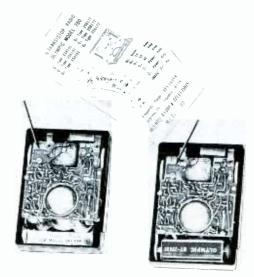
Fig. 5. Printed boards often contain numbers that can be used to match sets.
