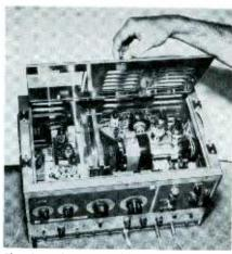
Fig. 2. B & K 1076 has many familiar TV circuits plus entire scanner system.
