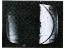
Fig. 1. Shadow blots out large part of raster, even at maximum brightness.
