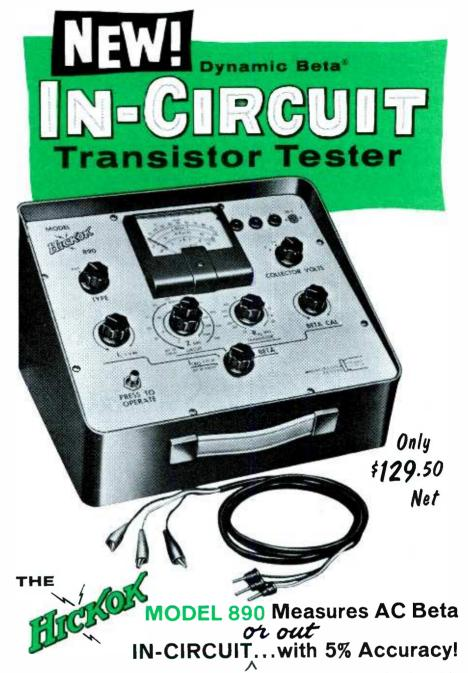
With the new Model 890, you can measure AC Beta-in circuit-with unmatched accuracy. The key to this new accuracy standard is the unique HICKOK-developed (patent-applied-for) method of neutralizing circuit impedance before tests are made. This effectively nullifies the loading effects of external circuit impedances and thereby eliminates the inaccuracies inherent in other methods.
