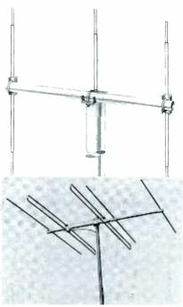
Three-element beam antenna—driven dipole flanked by reflector and director—has unidirectional reception pattern whether mounted horizontally or vertically. Additional parasitic (and driven) elements give beam or Yagi antennas higher gain, sharper directivity, and narrower bandwidth. Horizontal polarization is common in various point-to-point communications services.
