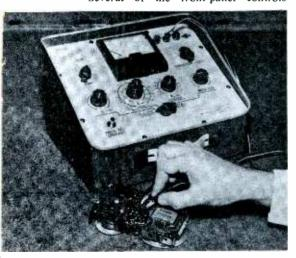
Fig. 4. The new Hickok Model 890 tests transistors either in or out of circuit.
