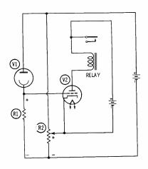
Fig. 2. A vacuum-tube amplifier used with DC-powered photoelectric tube.
