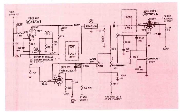
Fig. 3. Video amplifiers and noise-inverter stage of the RCA Chassis CTC7A.
