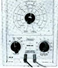
Fig. 5. Two switches and one control select all functions of the Substitutor.
