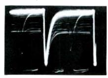
(A) Normal sync-pulse waveform.
