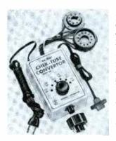
A multipurpose adapter newintroduced by Antronic Corp., the Anchor Model TC-438 "Chek-Tube Convertor," permits connecting either the 90° or 110° type of 8" check tube to a CRT socket designed for either the conventional 12L duodecal base or the 8HR standard 110° miniature 8-pin base. In addition, a selector switch sets up the proper base connections and power ratings for substitution testing of five groups of CRT's having unusual filament characteristics. Price is \$11.95.
