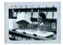
Finished guns after ultrasonic cleaning in a super wetting agent are carried to the assembly line in these covered plastic cases -further protection against contamination.
