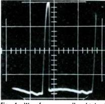
Fig. 4. Waveform normally obtained when scope probe is attached to 1B3.
