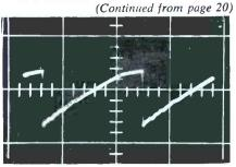
Fig. 2. The flattened grid waveform at the output tube held the first clue.
