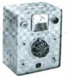
A continuously-variable output from 0 to 140V AC, isolated from the 120V input, is furnished by **Standard Electrical Products'** "Adjust-A-Volt" IV Series transformers. Capacities range from .28 to 4.8 KVA. Deluxe units in portable cases, with output voltmeter and thermal circuit breaker, are made in three sizes; there are also two sizes of uncased units for builtin in stallations.
