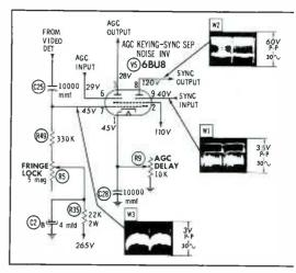
Fig. 4. Zenith Chassis 16F25 has a typical 6BU8 noise limiter circuit. more negative than ground. Since the delay voltage from point A is minimum at this time, a negative voltage begins to appear on the RF-AGC line soon after the IF-AGC voltage passes through zero.
