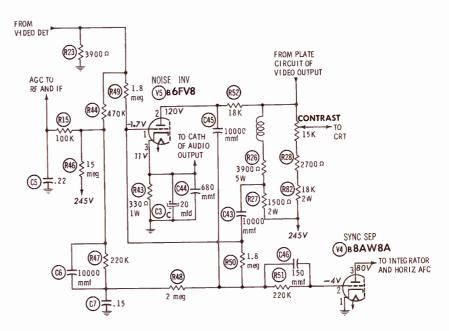
Fig. 3. Westinghouse V-2384-15 has different version of triode circuit.
