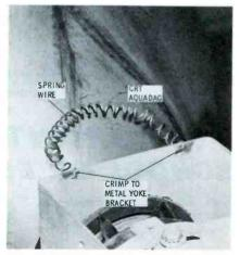
Fig. 2. Improvising a ground for the aquadag coating is no real problem.
