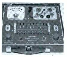
Fig. 8. Front panel of Model 85 has no roll chart; setup data is in booklet.
