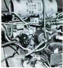
Fig. 1. CRT substitution may involve the addition of a high-voltage filter.
