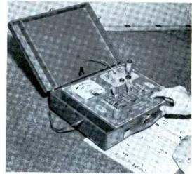
Fig. 7. Superior Model 85 checks the tubes for shorts, leakage, and quality.
