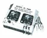
The SENCORE Model BE113 "Align-o-pak," a dual version of the Model BE3, is designed to supply two individually-variable negative DC voltages for AGC clamping and similar applications. The output from each section of this ACpowered unit ranges from 0 to 20 volts with less than 0.1% ripple. Dealer net price is \$12.75.
