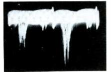
(C) Pin 7—R5 advanced. Fig. 5. Noisy signal fed to 6BU8.
