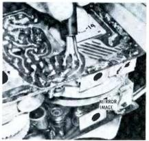
(A) For in-circuit transistor test.
