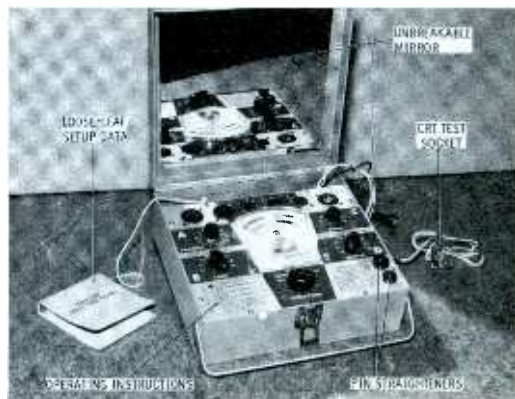
Fig. 8. A number of "extras" are found on the new Mighty Mite tube tester.
