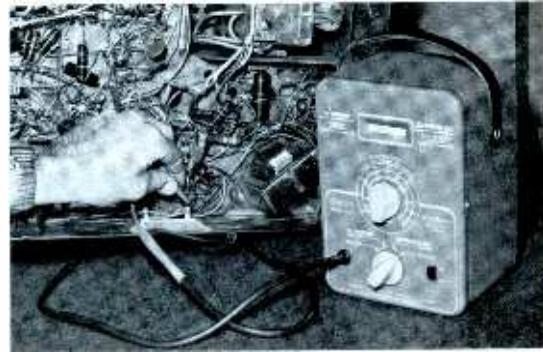
Fig. 4. In-circuit tester detects bad capacitors with low shunt resistance.
