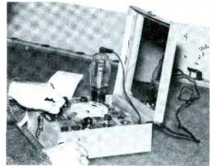
Fig. 7. SENCORE'S Model TC109 features a highly sensitive grid-leak test.
