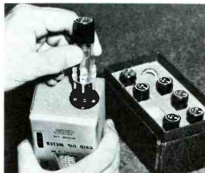
Fig. 2. Model 710 plug-in coils cover frequencies from 400 kc to 250 mc.
