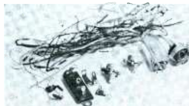
Fig. 2. These burned parts were replaced after complete check of chassis.
