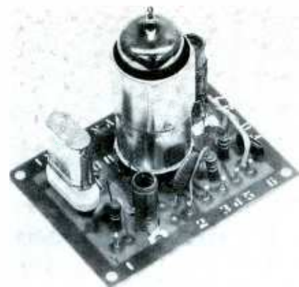
Fig. 5. RF stage of CB transmitter on small plug-in printed wiring board.
