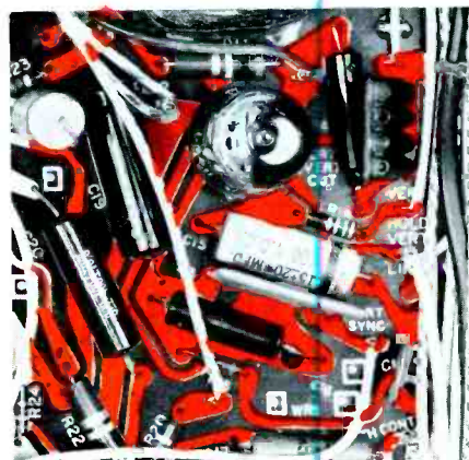
Fig. 4. Lines on Philco board show exact paths of foil conductors between components. Many tie points are named.
