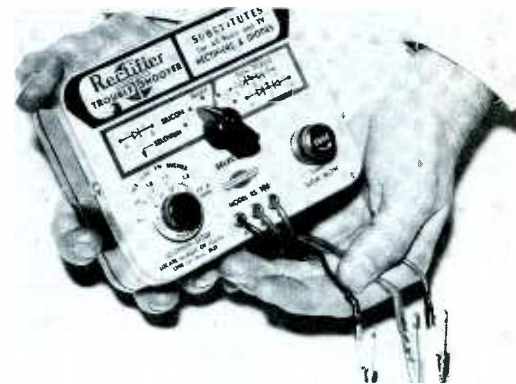
Fig. 3. A new substitution instrument for locating bad diodes and rectifiers.
