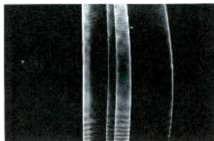
(A) Dim, badly-distorted raster.
