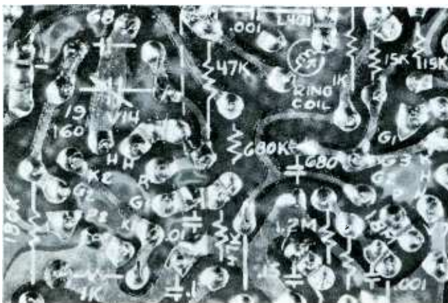
Fig. 1. Schematic symbols on Westinghouse See-Matic board facilitate circuit-tracing from conductor side.
